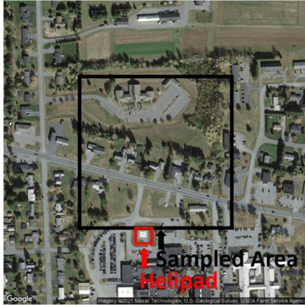
Figure 1: Sampling images from Google Earth for building datasets of positive (helipad is present) and negative examples (no helipad is present). The dataset will be used to train machine learning and AI models. The sampled area is enclosed in the black box. There is no helipad inside the sampled area (negative example). However, a helipad is present just outside the sampled area. The area containing helipad can be also be sampled as a positive example.
