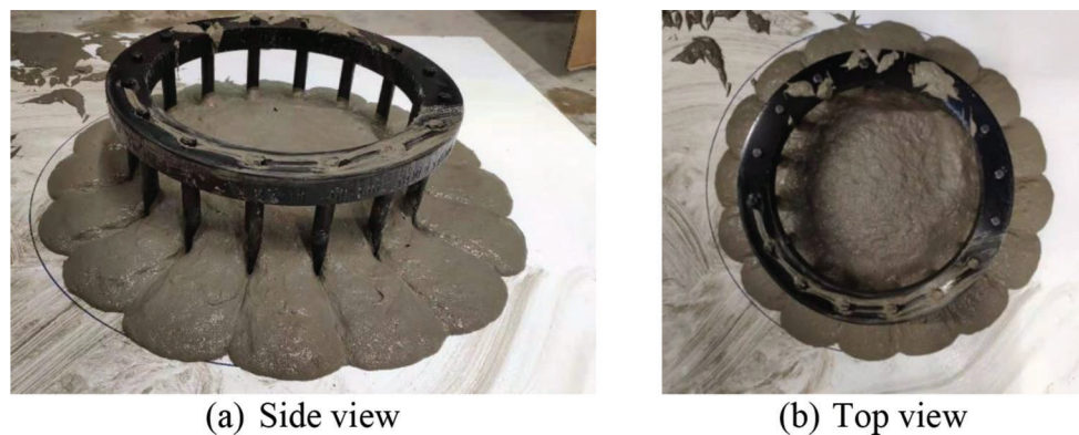
Figure 7.1 Set up and results of SHCC J-ring testing.
