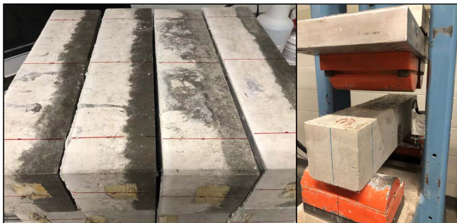
Figure A.17 SHCC sample and flexural testing.
