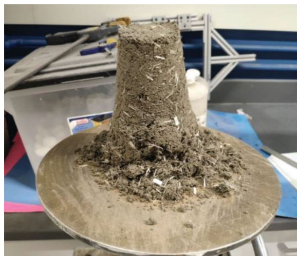
Figure 5.3 Mini-slump test for SHCC with 0.664% SAP.
