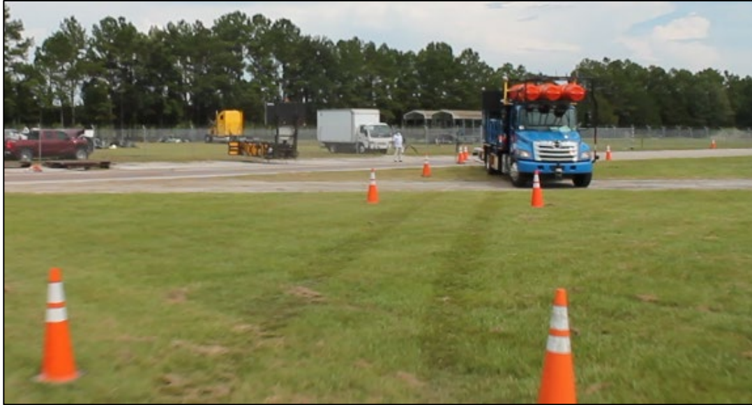
Figure 6-65. External camera view of follower truck turning. The follower vehicle unexpectedly leaves its course.
