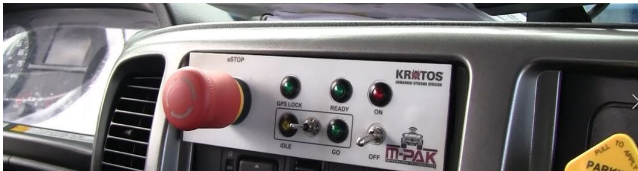
Figure 3-14. Follower truck – Internal controls: In the center of the dash is the follower truck version of the operator control unit (OCU). Near the right of the panel is the on/off switch which engages the OCU in preparation for autonomous operation. The light above the switch verifies that the system is on and operational. When the OCU is switched on, the system will attempt to locate GPS signals. When 6-7 satellite signals have been located, the GPS Lock light illuminates. When the system is powered on, initialized, and GPS lock is achieved, the Ready light lights up to show that the follower vehicle is ready for autonomous mode. The switch in the black rectangle switches the follower vehicle between idle mode and GO mode: in idle mode, the follower truck is ready for autonomous mode but still under manual steering, braking, and accelerating control; in GO mode, the follower truck is in autonomous mode and under control from the leader truck. When leader driver has completed the leader vehicle checklist, the follower driver will be instructed to enter “Go” mode, and the GO light illuminates. The follower driver will then exit the follower vehicle and enter the passenger seat in the leader vehicle to act as system monitor. The follower driver can return to the follower vehicle at any time it is stopped, switch to idle mode, and take manual control of the follower vehicle. The big red button on the OCU panel is an E-stop (only active when the OCU is on). An E-stop will be activated automatically if the follower vehicle loses contact with the leader.
