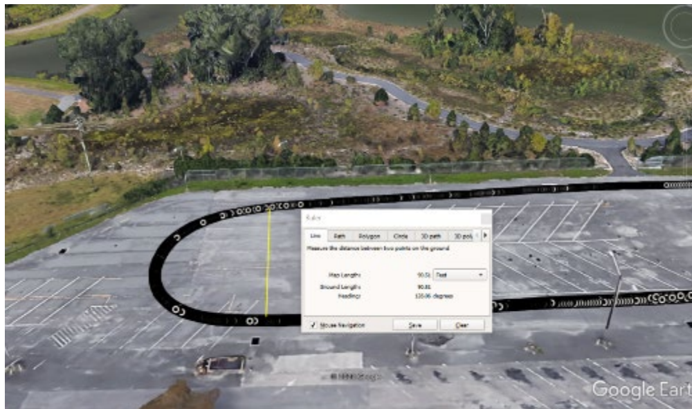
Figure 6-63. Trajectory from log file results that shows two of the successful turns with radius of 45 ft
