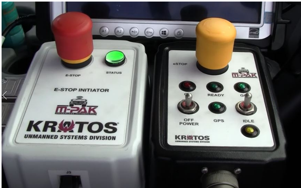
Figure 3-20. The control panels are the same as the dashboard OCU panel in the follower truck. On the left is an E-stop activator. On the right are the on/off and idle/GO switches and the GPS Lock and Ready lights. The big yellow button is an A-stop.
