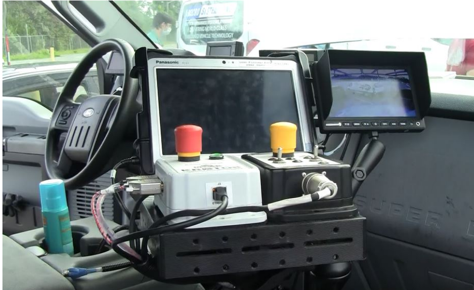
Figure 3-19. The leader vehicle OCU includes a laptop computer screen that displays the control user interface, two control panels in front of the screen, and a viewer that displays the signal from the follower truck's front-facing camera. The OCU is held on a pivoting arm that is pulled out for a clearer view. Through the user interface, the follower truck operator can enable the system, view warnings, adjust offset and gap, and more.
