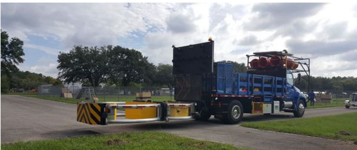
Figure 3-7. Follower vehicle showing Scorpion impact-absorbing device extended to the rear
