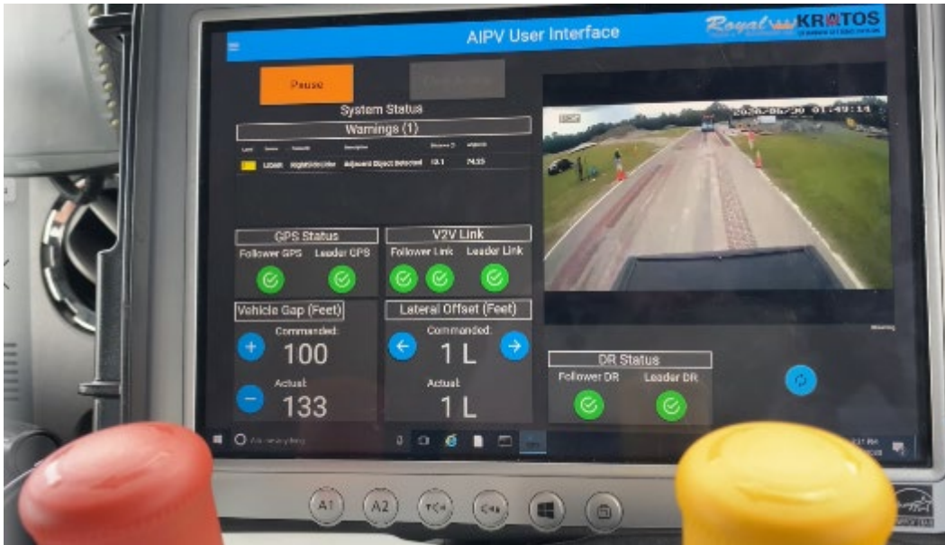
Figure 6-56. User interface view of lateral offset test showing 1-ft offset towards left
