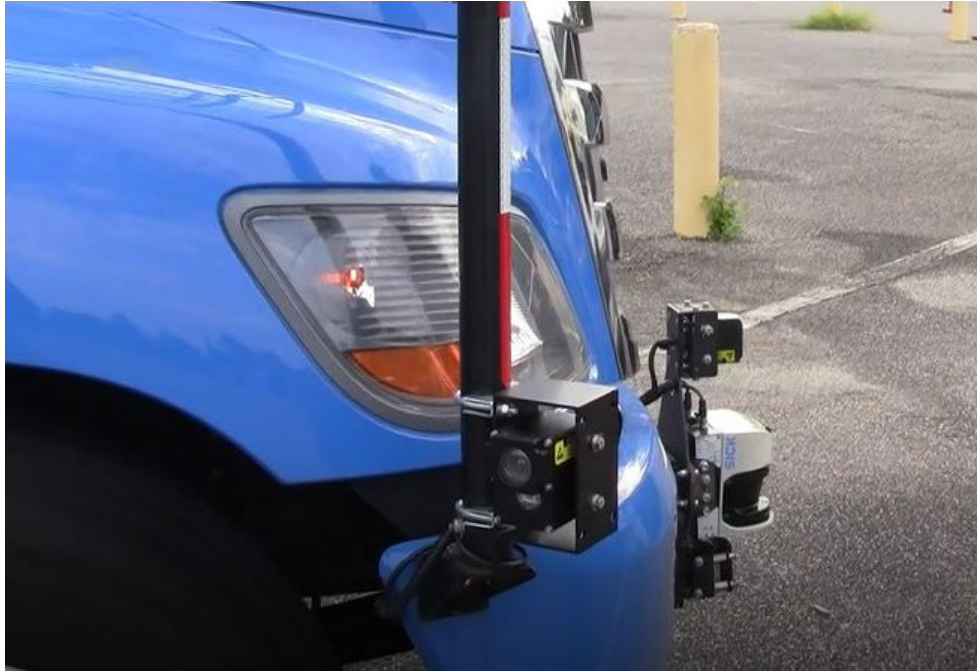
Figure 3-9. Follower truck – External sensors: In the lower center of the image is the lateral-facing lidar. There is one on both sides of the follower truck. It has a field of view of 100° to 120°. If an object is detected, the person in the leader vehicle monitoring the follower vehicle is notified by through the user interface, but it will not cause an A-stop. The mount is readily adaptable to many vehicle types.
