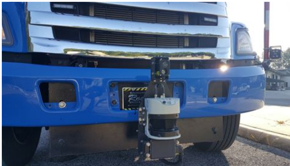
Figure 3-8. Follower truck – External sensors: The forward-facing obstacle detection system is attached to the front bumper of the follower vehicle. (1) The large device in the white housing is an off-the-shelf lidar (SICK, Inc.) which has a 190° view. During autonomous operation, the lidar narrows its field of view to the leader vehicle so that during a turn or in a roundabout, the follower vehicle will not respond to objects that are in its line of sight but not in its path of motion. Otherwise, the follower vehicle would detect, for example, a street light on the opposite corner and execute an automatic stop (A-stop). (2) The rectangular black device below the white housing is a standard automotive radar (Delphi, Inc.). The radar can detect objects out to 150 ft. If the radar detects an object in the range of 100 ft to 150 ft, the follower truck will automatically slow to 7 mph. If the radar detects an object within 100 feet, the follower truck will execute an A-stop. (3) The lensed device above the white lidar housing is a legacy lidar. It is no longer used and will be not be included in future versions of the system.
