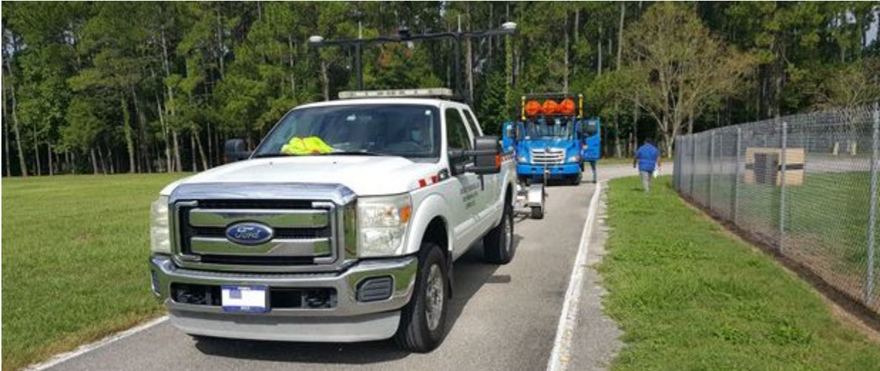
Figure 3-6. ATMA trucks in demonstration configuration. The white truck in the foreground is the FDOT F350 truck retrofitted with the Kratos leader kit. In the background in the blue follower truck, rented from Kratos.
