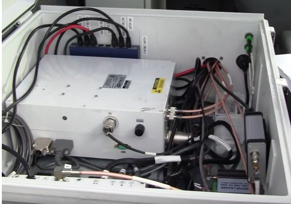
Figure 3-21. Leader vehicle: System hardware – “The brain of the system” is located behind the passenger seat. It draws power from battery as shown previously and includes the GPS receiver, interfaces to the OCU and I/O computer, the vehicle interface, radios, fiber optic gyro, and receiver for analog video.
