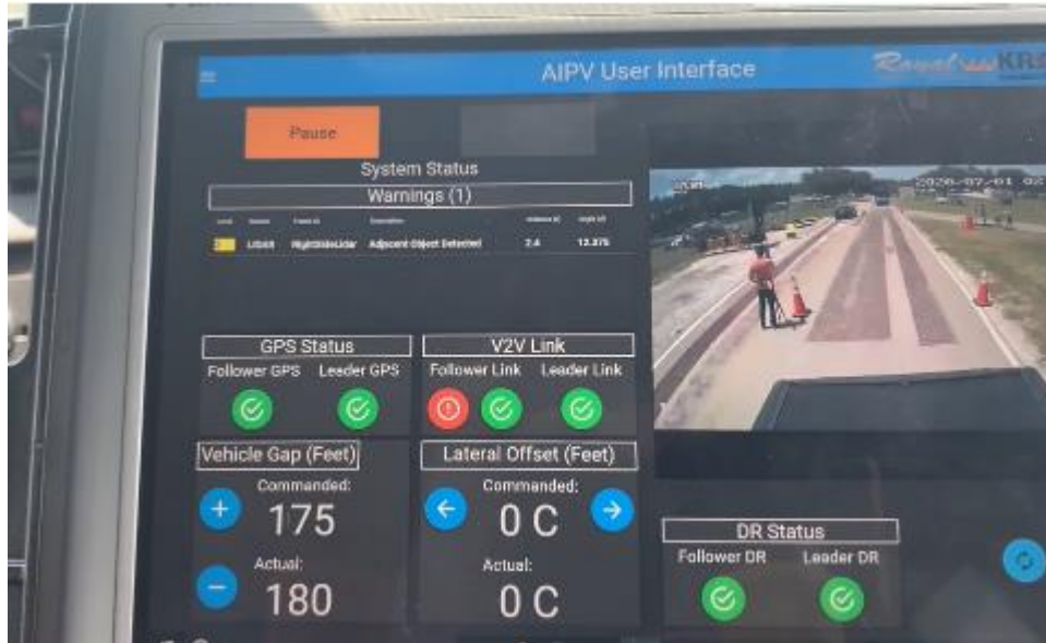
Figure 6-90. User interface view showing the warning as it recognized the object
