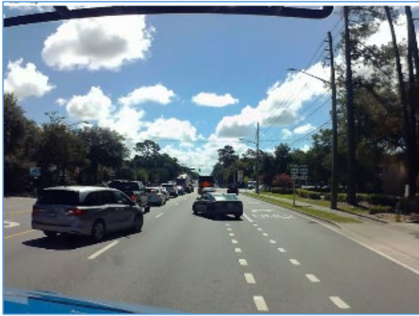
Figure 6-115. Multiple vehicle intrusions in front of ATMA that caused frequent A-stops
