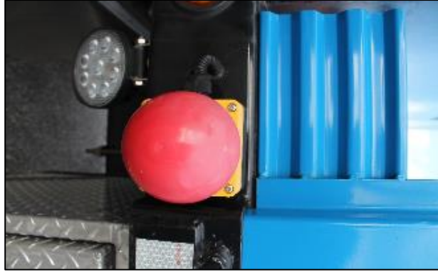
Figure 6-3. Emergency stop ATMA follower external button
