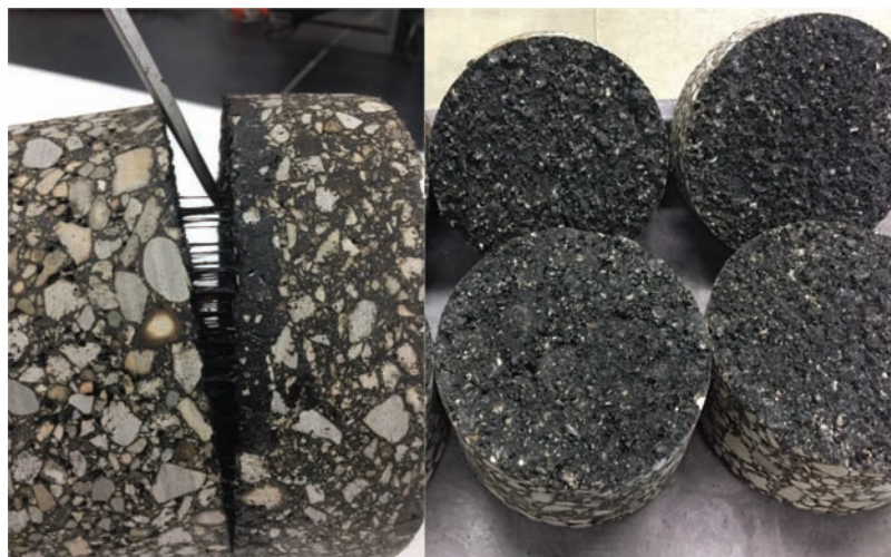
Figure 3.5 VRAM specimen (left) and SS-1h (right) after failure.
