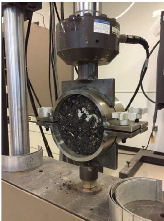
Figure 2.2 Shear apparatus in MTS machine.
