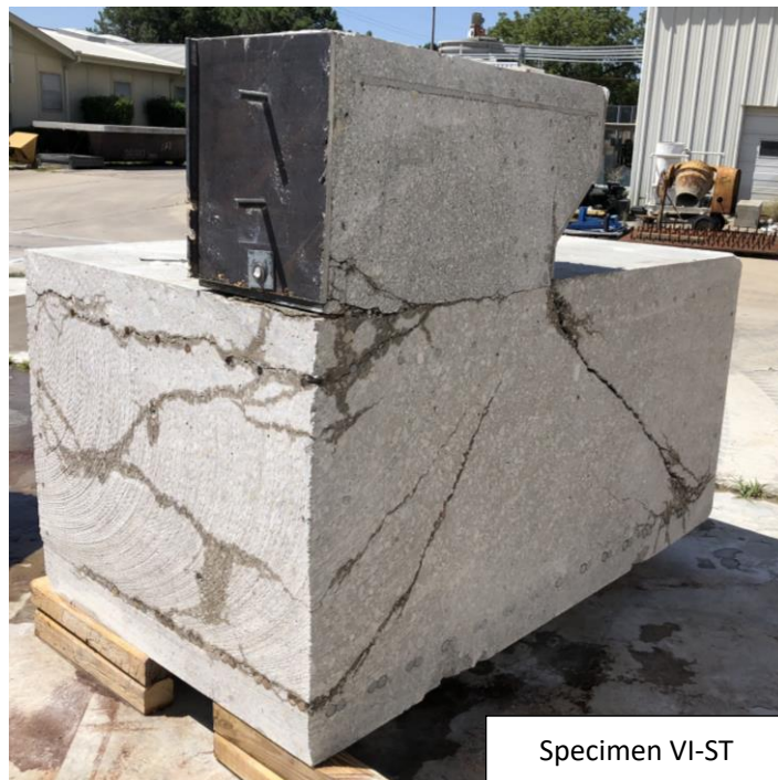
Figure 5.18 Internal cracks formed entire with of specimen (VI-ST)
