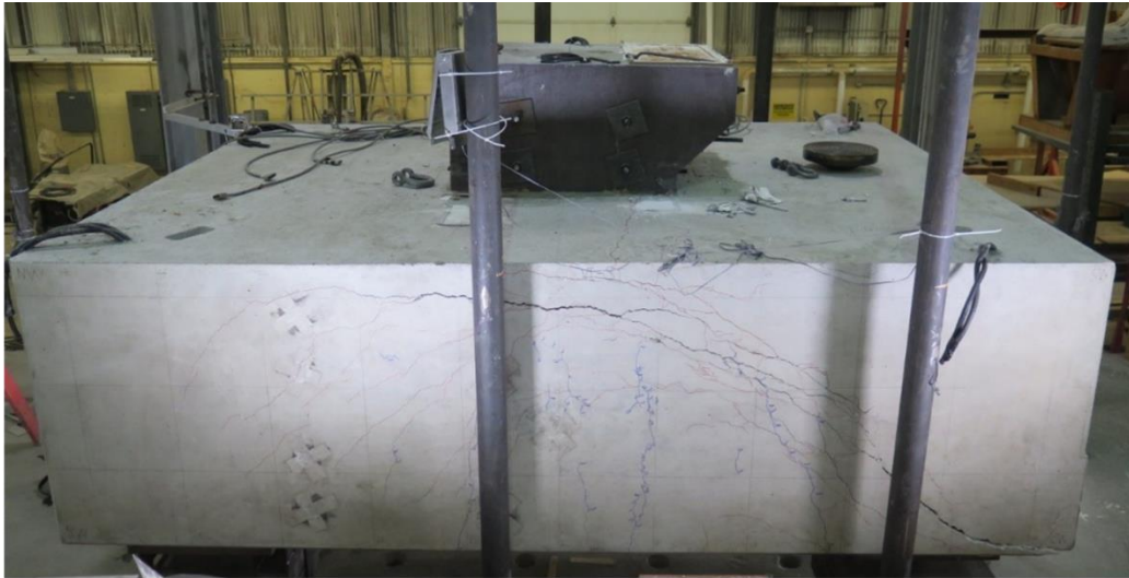
(a) Damage on side surface of footing (west)
