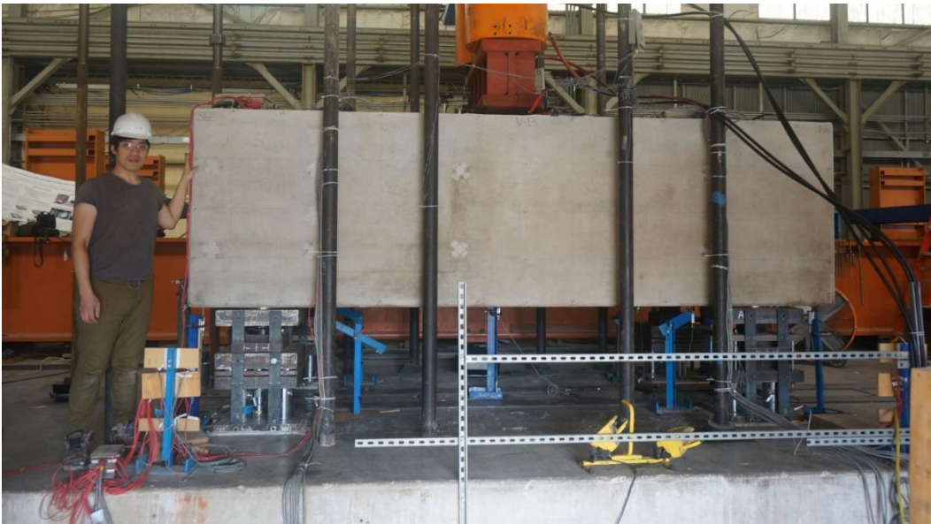
Figure 4.25 V-13 after setting up the loading test
