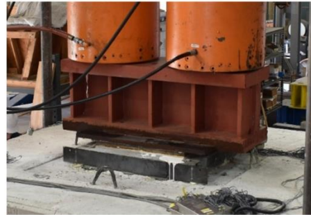
(b) Spreader beam after setup
