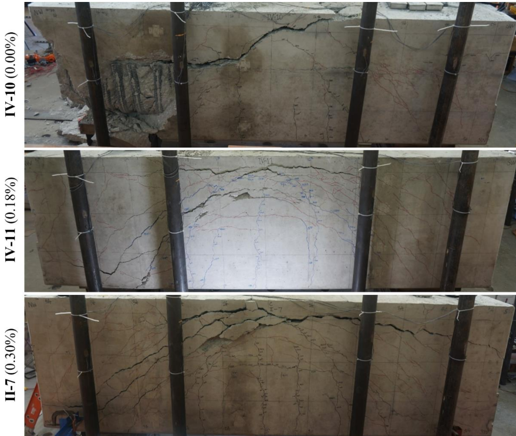
Figure 4.46 Comparison of post-failure conditions on the side faces between specimens: Series IV
