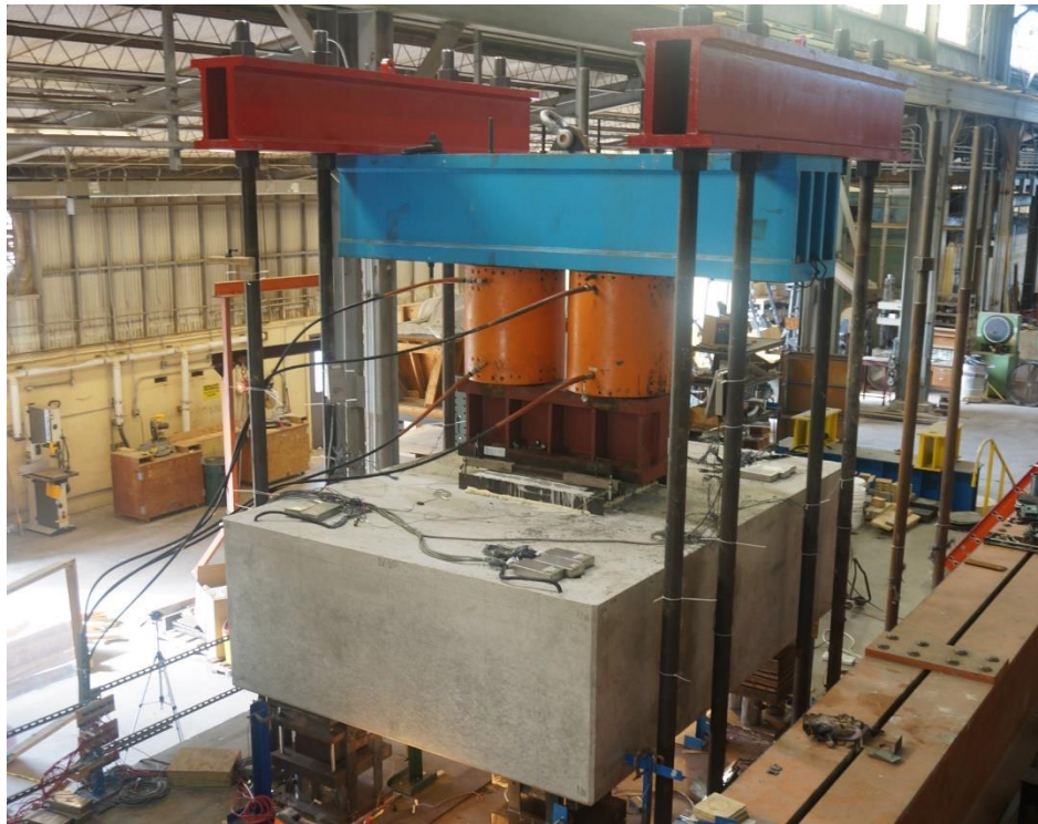
Figure 4.10 Structural test setup
