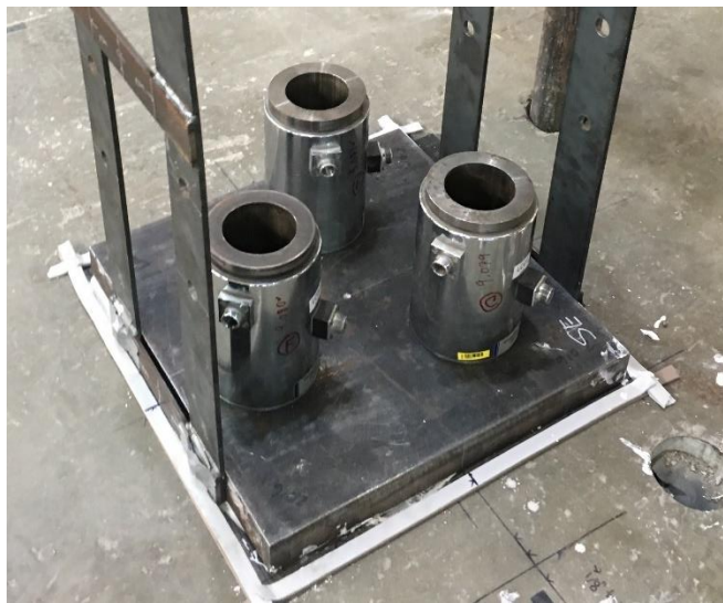
Figure 4.28 Load cells in the support fixtures
