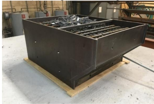
(d) Install the steel jacket with the 0.5-in. gap (plywood)
