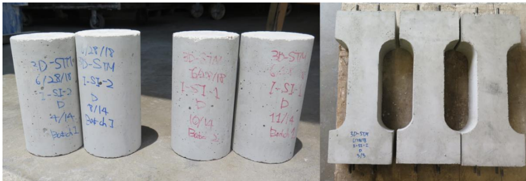
Figure 4.7 Concrete cylinders (left) and dog-bone direct tension specimens (right)
