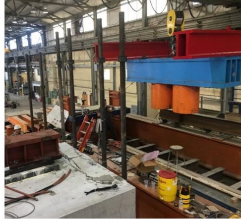
(b) Loading frame during Installation
