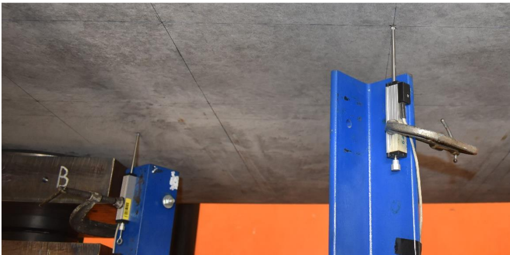
Figure 4.29 Linear potentiometers to measure displacements on the bottom surface
