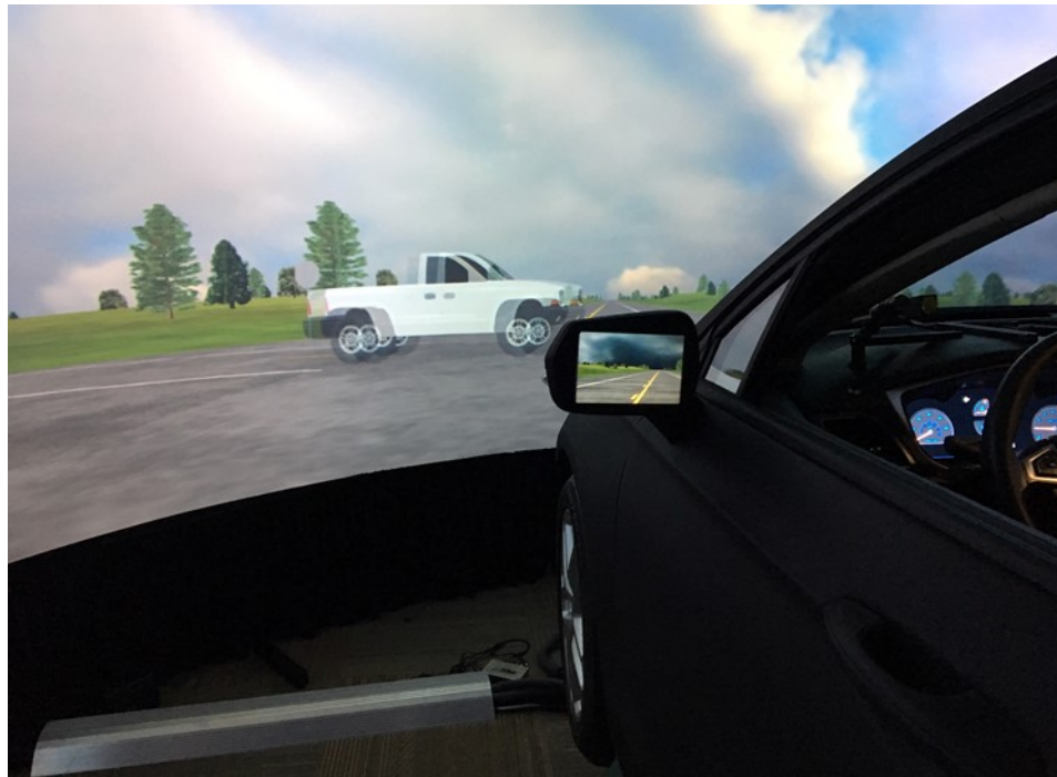
Figure 3.2. Image of moving pickup truck crossing participant vehicle in the sight estimation test.
