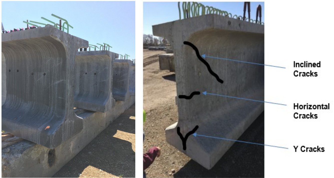
Figure B-1: Web cracking observed during the production of current MnDOT girders. (Left: MN45 at County Materials in Roberts, WI Right: MN45 at Forterra in Elk River, MN)
