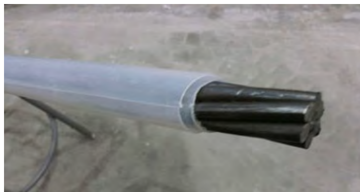
Figure 1-3: Strand debonded with flexible split-sheathing tube
