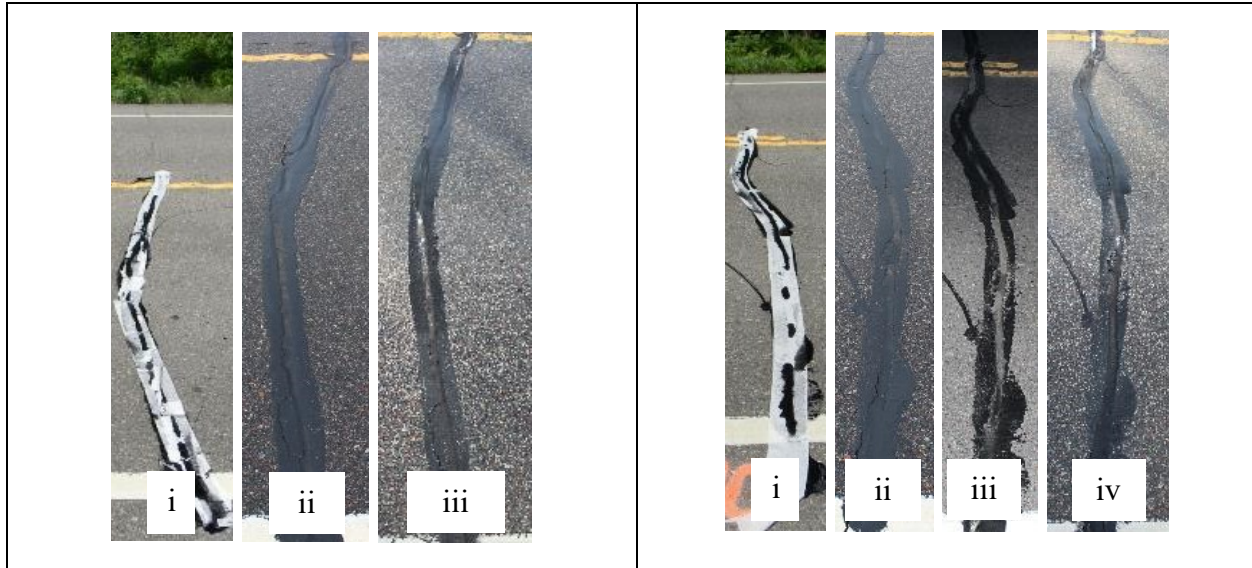
Photographic Performance Documentation of Site E. E-1-i Shows Crack E-1 upon being sealed. E-1-ii and E-1-iii shows Crack E-1 at the end of its first winter and during the second winter after being sealed. This same sequence of photos follows for cracks E-2, E-3, E-4, E-5, E-6, E-7, E-8, E-9, and E-10. E-10-iv shows the seal performance at the end of the first winter compared to the mid-winter performance presented in E-10-iii.
