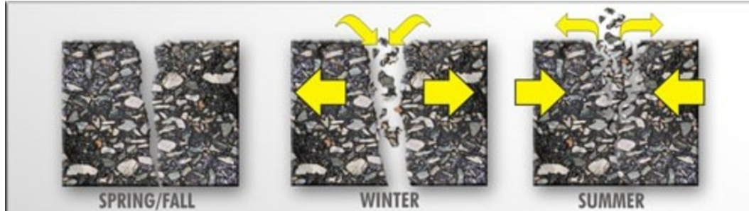
Figure 2.2: Incompressibles Intrusion Related Damage (after, Stoikes, 2017)
