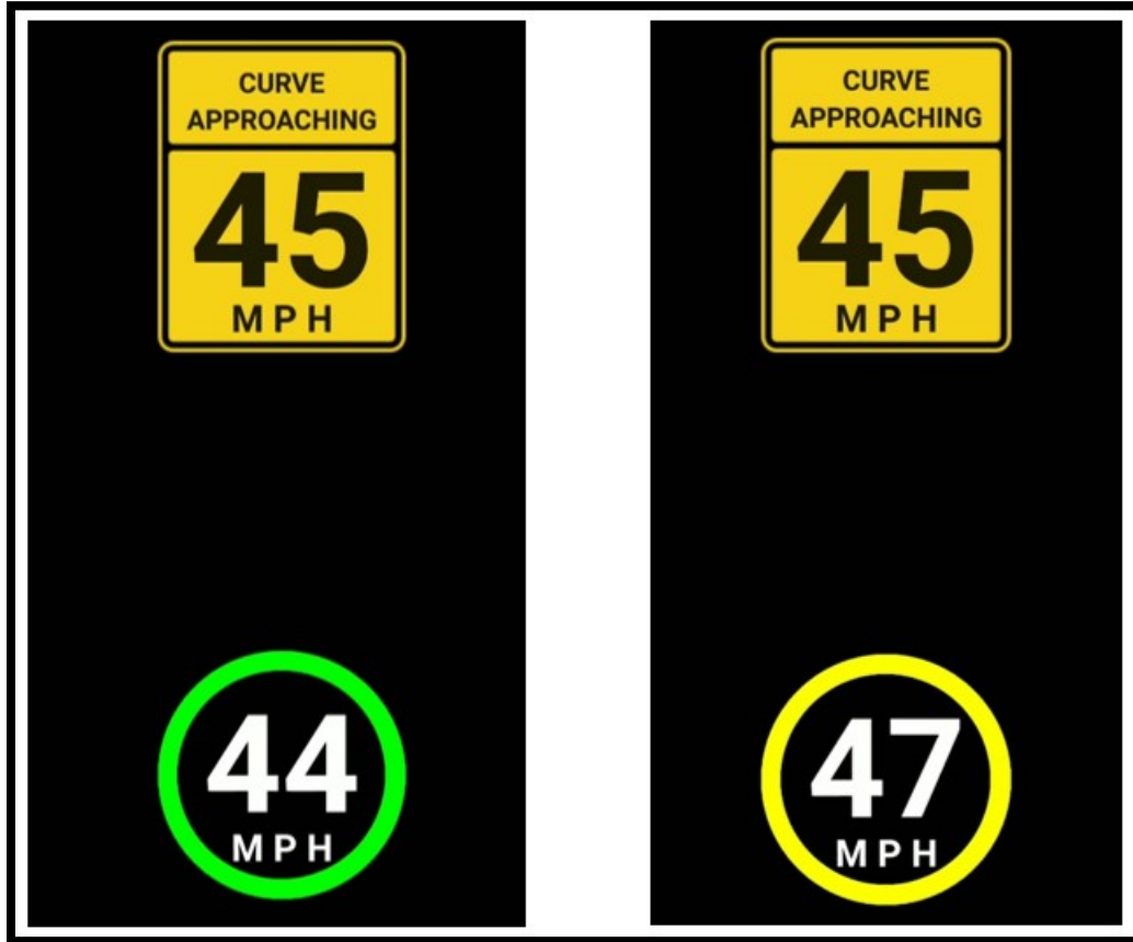
Figure 3.3 Initial warning display for traveling at or below the advisory speed (left) and above the advisory speed (right).
