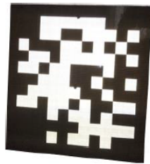
Retroreflective 2D code in visible light Black printing on white sign sheeting
