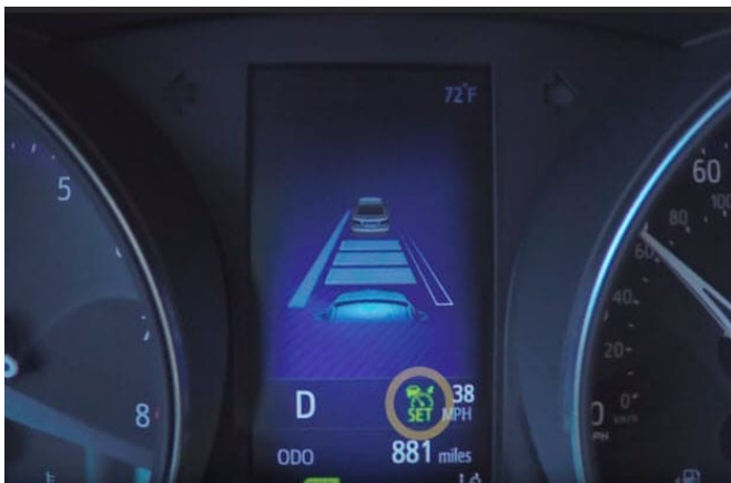
Figure 2-3. Dynamic radar cruise control
