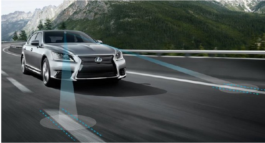
Figure 3-1. Use of cameras and image processing to identify lane lines
