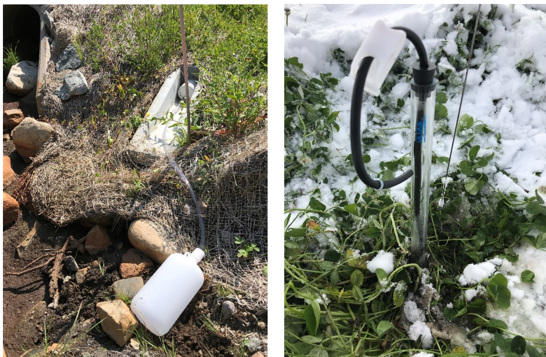
Figure 6.27. Leachate collection from Eagles Nest trench (left) and lysimeters installed in Eagles Nest slope (right).
