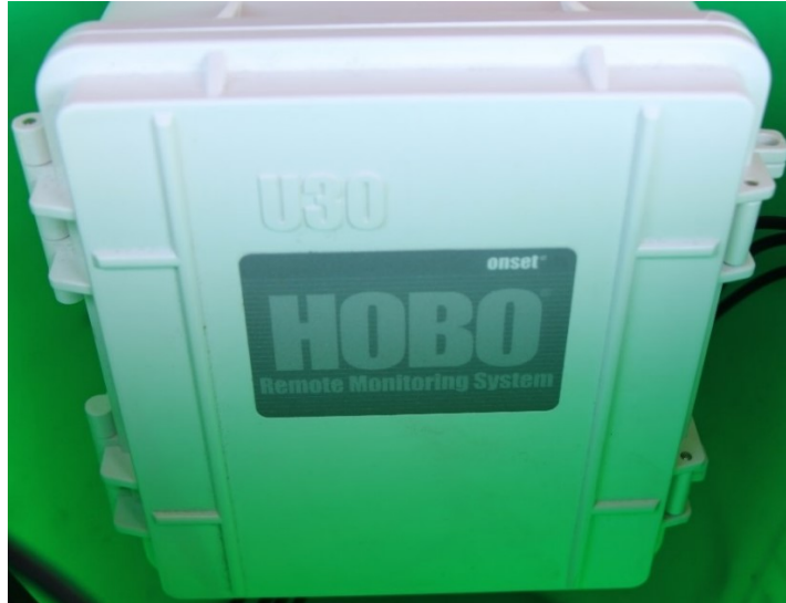
Figure 6.7. Data acquisition unit used to record soil moisture, rainfall and temperature during monitoring.
