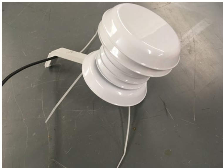
Figure 6.10. Temperature probe with solar shield.
