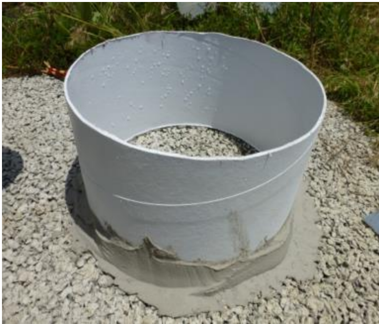
Figure1. Infiltration Test setup
