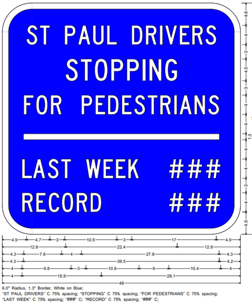
Figure 3.9 Feedback Sign Dimensions (credit HunWen Westman, P.E., Saint Paul Public Works)
