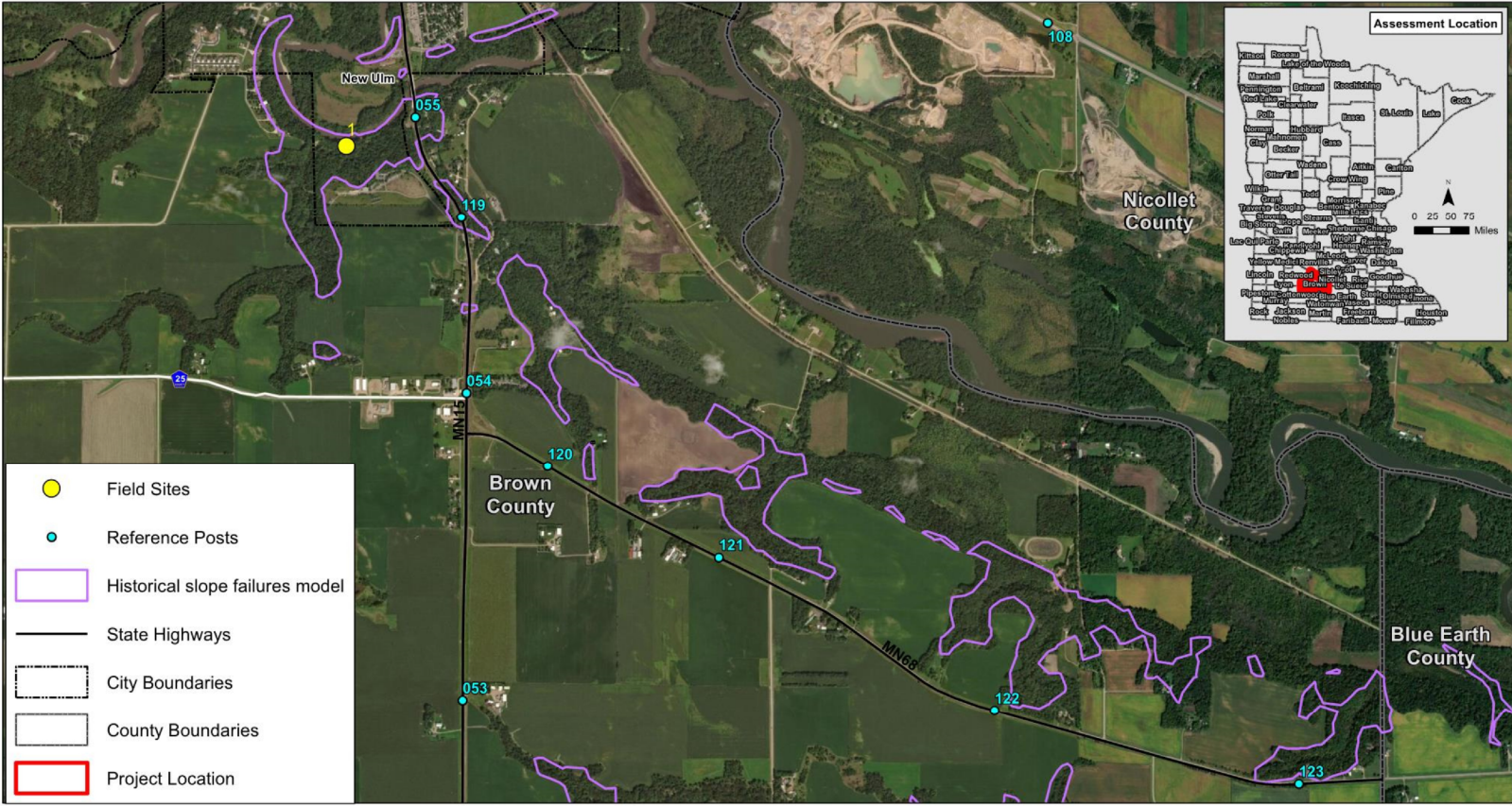
Figure 10. MnDOT Field Assessments Site 1 - MN-68, Brown County, District 7 Historical Slope Failures (Model Part 1)
