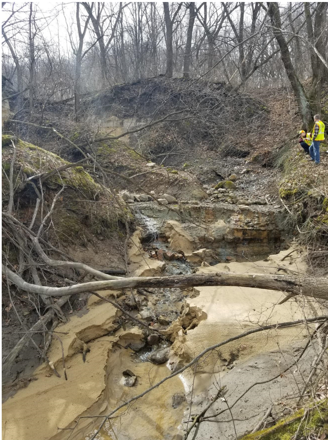
Figure 15. Intersected Water Table/ Spring. Photo: Nick Bradley, WSB.
