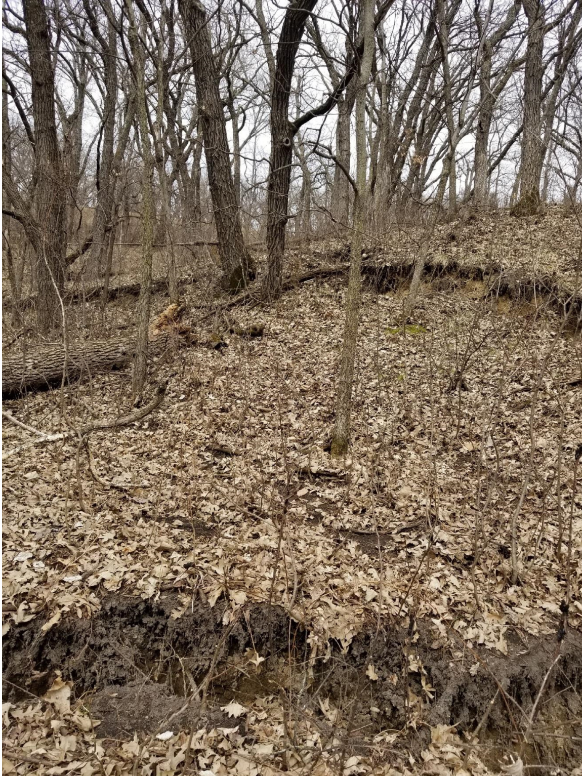
Figure 21. Dozens of scarps formed around the same time spanning from the river to the higher road surface 500 feet away. Photo: Nick Bradley, WSB.
