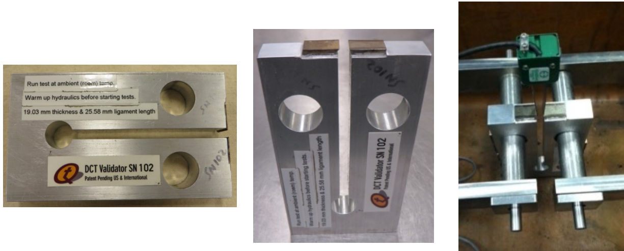
Figure 4-1 MnDOT Approved Validator and Validator Loaded in DCT Testing Chamber
