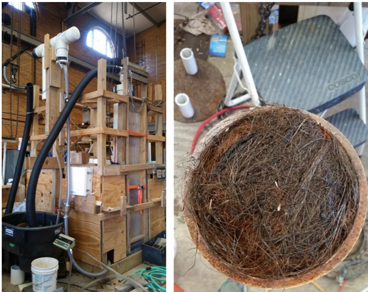
Figure 6 Permeameter (left photo) and Conductivity Chamber (Coir, right photo).
