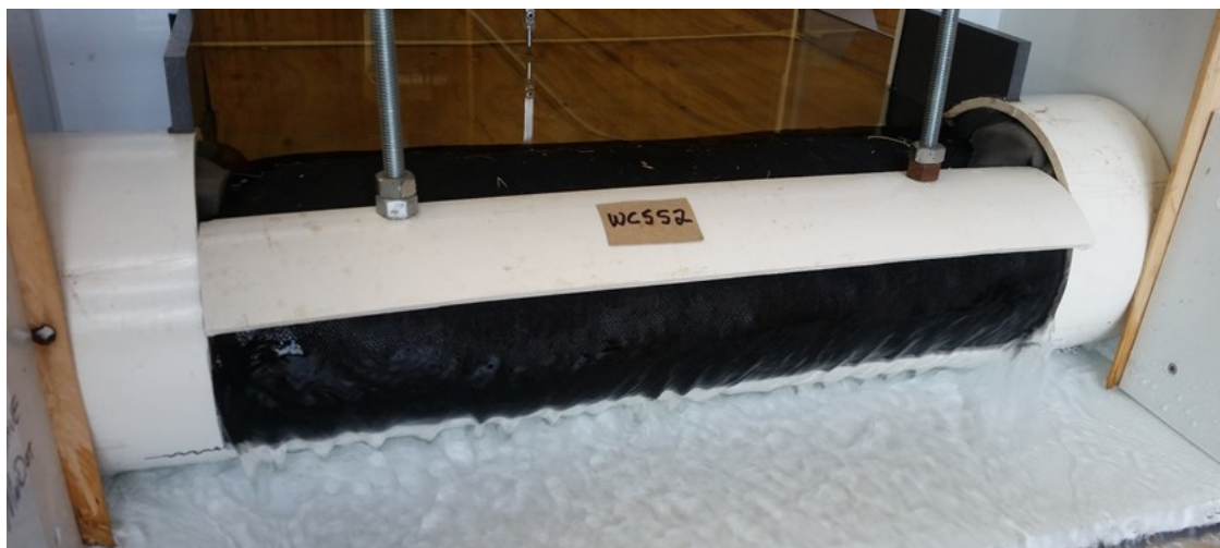
Figure 2 Sediment Control Log with Wood Chips (WC Red, Eco-Guard Compost ).
