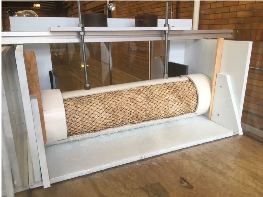
Figure 8 Frame Attachment and Log Holder for Flume Studies.
