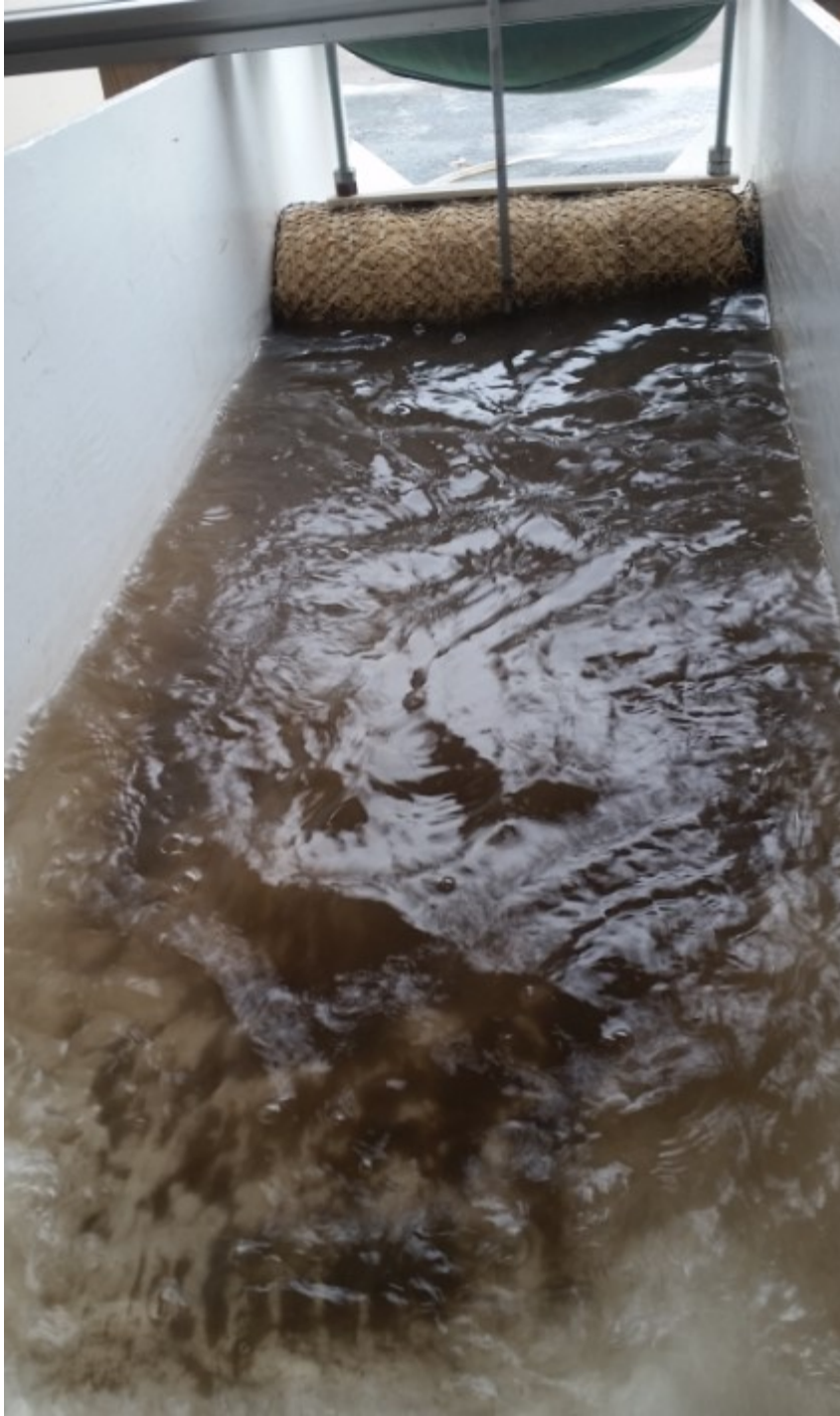
Figure 13 Facing Downstream, Log Holder for Sediment Flume Studies.
