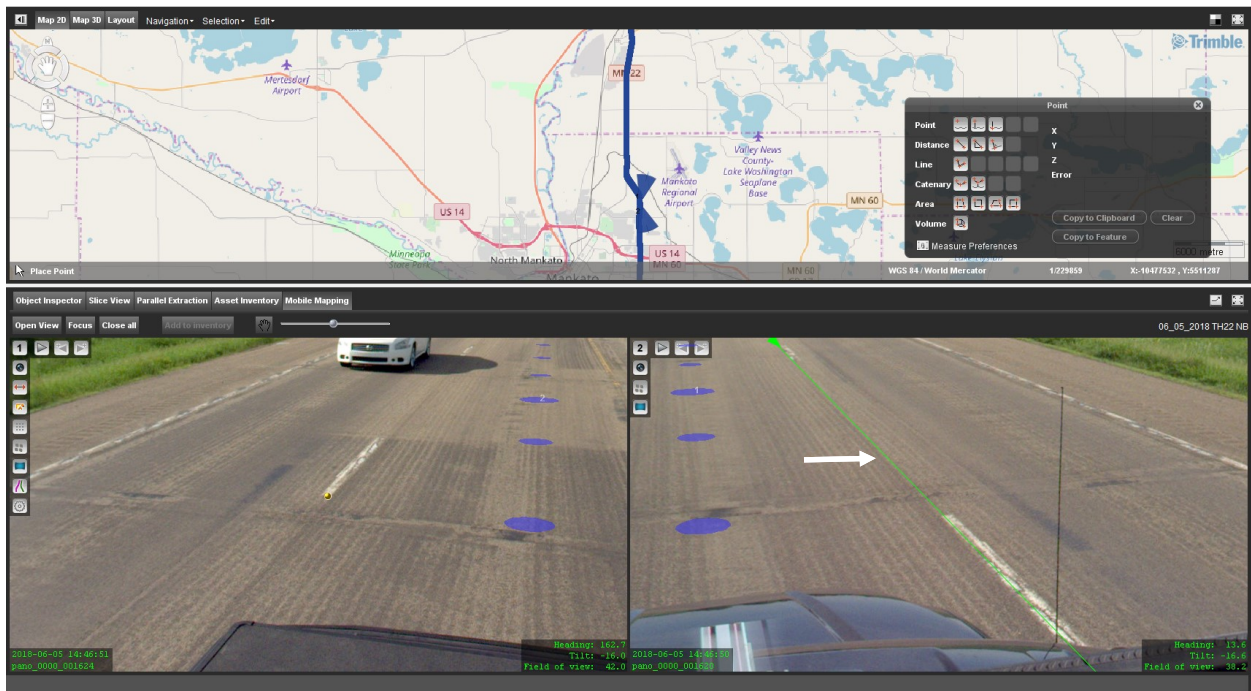
Figure 3.9 Image of the creation of the centerline feature using the forward intersection method.
