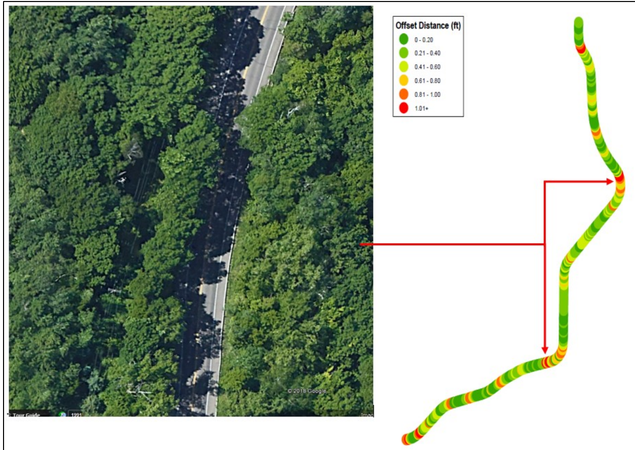
Figure 3.17 Plan view map of Trimble MX7 higher position error under tree canopies (TH3, forward intersection extraction).
