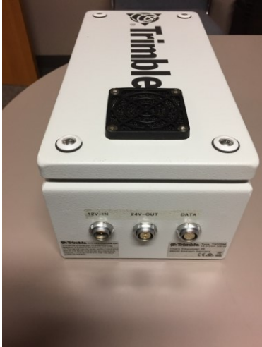
(c) Power Conversion Unit – 3 ports for 12V in 24V Out data.
