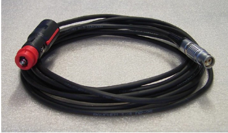
Figure A.8 Photo of power cable to be connected between power converter unit and vehicle.
