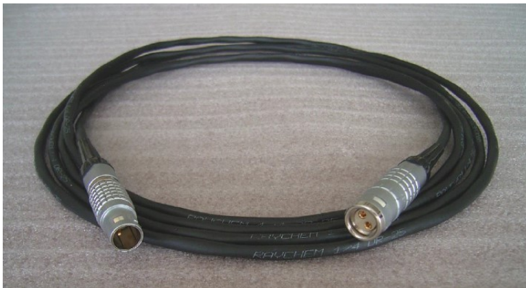
Figure A.4 Photo of power cable to be connected between the MX7 and power converter unit.
