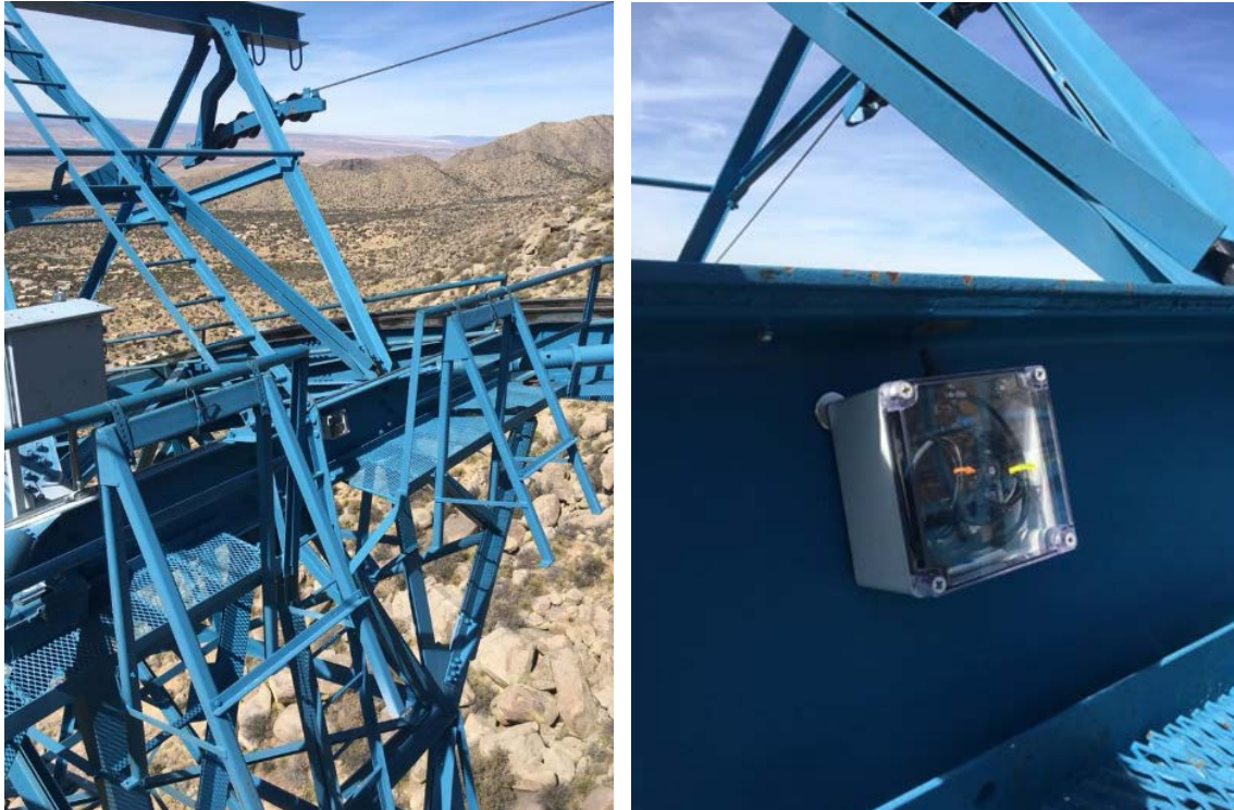
Figure 34. LEWIS 2 was placed in Tramway Tower to capture acceleration and angular velocity.
