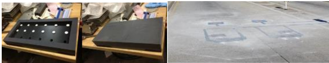
Figure 12. The prototype and pattern of In-situ Energy Harvester Placement (32)
