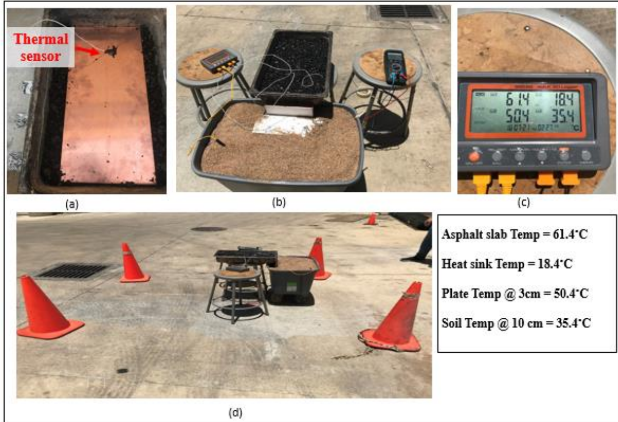
Figure 20. Field installation and data collection.
