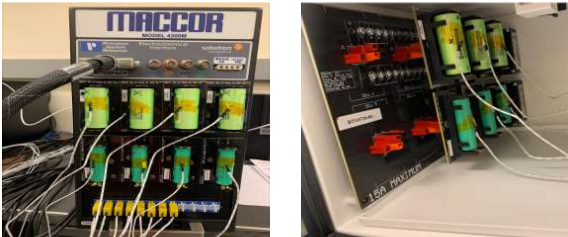
Figure 7. A123 26650 and 18650 Li-ion batteries (a) outside the environmental chamber at room temperature and (b) inside the environmental chamber with controlled temperature.
