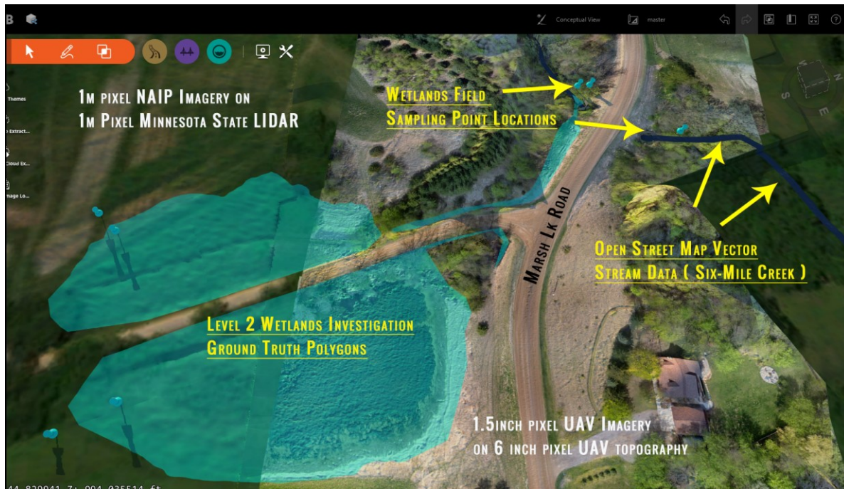
Figure 3-19: Screenshot illustrating stylized GIS wetland delineation polygons combined with other GIS data.
