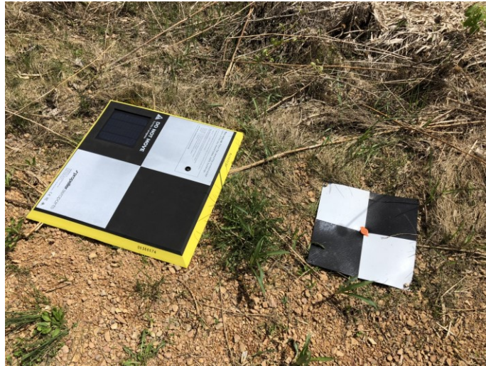
Figure 2-5: Comparison of Propeller Aeropoint (left) and Carver County-provided Aerial Control Point.
