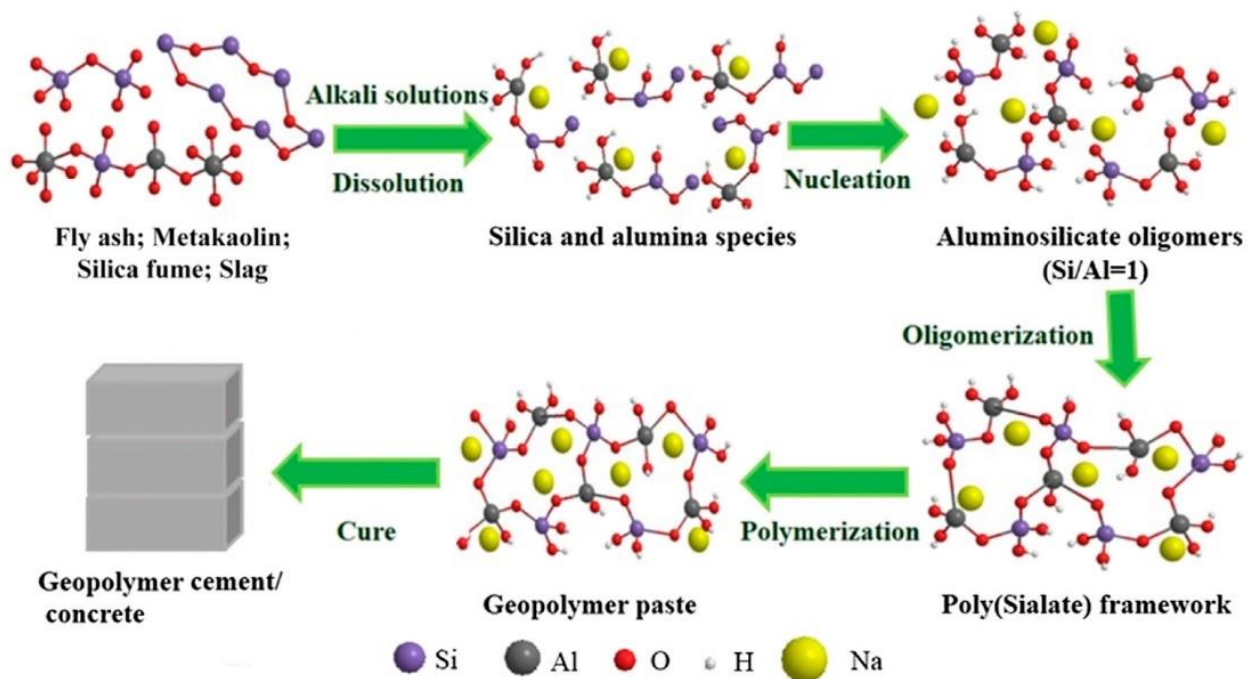
Figure 4. Reaction mechanism of geopolymerization.
