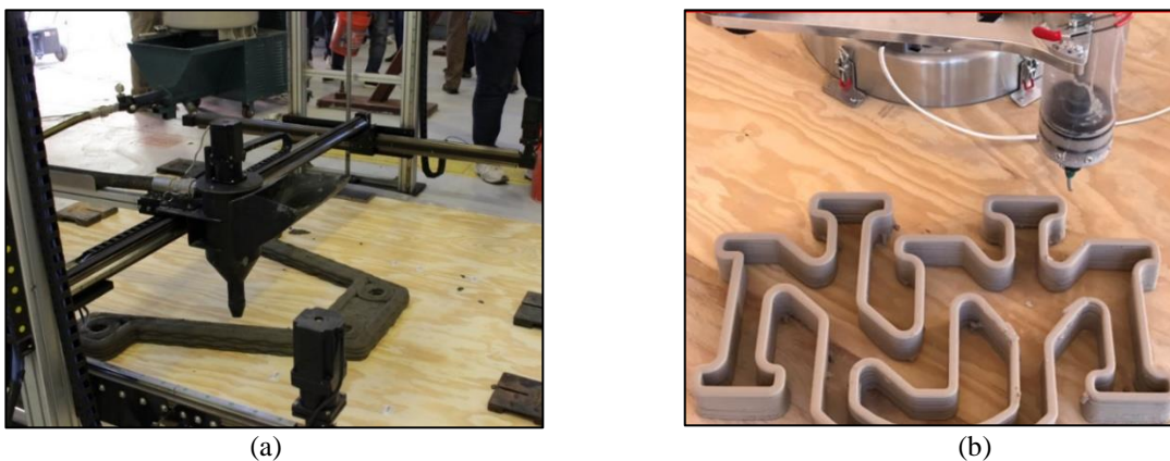
Figure 2. UNM Dana C. Wood Materials and Structures Lab 3D-Printing Systems (a) 3D-Printing of Concrete (b) 3D-Printing of Clay
