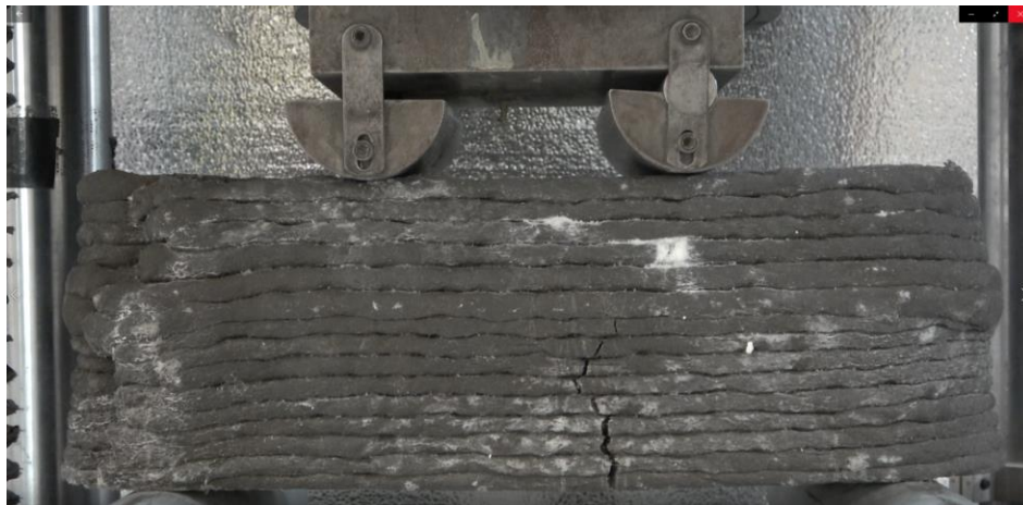
Figure 30. Single crack of the beam samples under flexural load.
