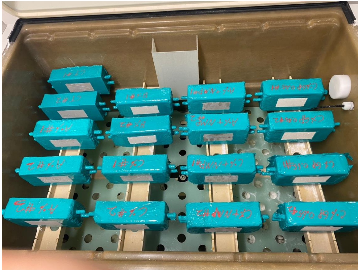
Figure 8. Fog-chamber testing under ASTM B117.
