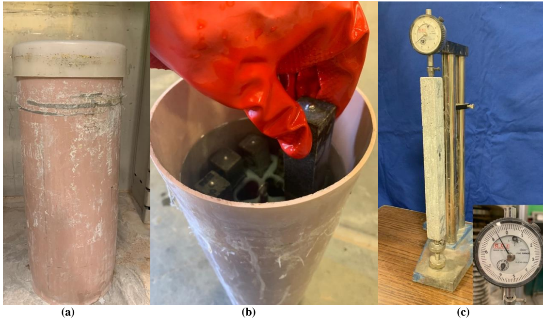
Figure 1. ASR Testing: (a) storage container, (b) removing sample from sodium hydroxide solution to take a reading, (c) dial gauge length comparator.
