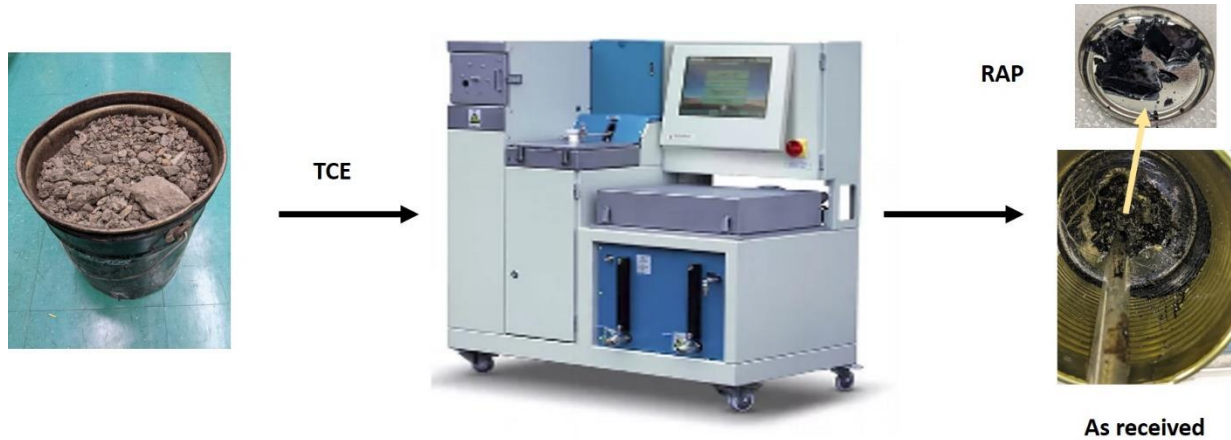
Figure 4. RAP samples extracted from aggregates using InfraTest™ Asphalt Analyzer.
