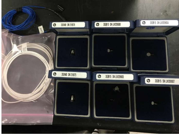
Figure 7. The accelerometer used for preliminary test in Task 2 to choose which bridge is the best field test location from candidates. The accelerometer made from PCB corporation (model number: 353B15). As a preliminary test, before selection of bridge, the team will do test in different bridges to make sure to get signal.
