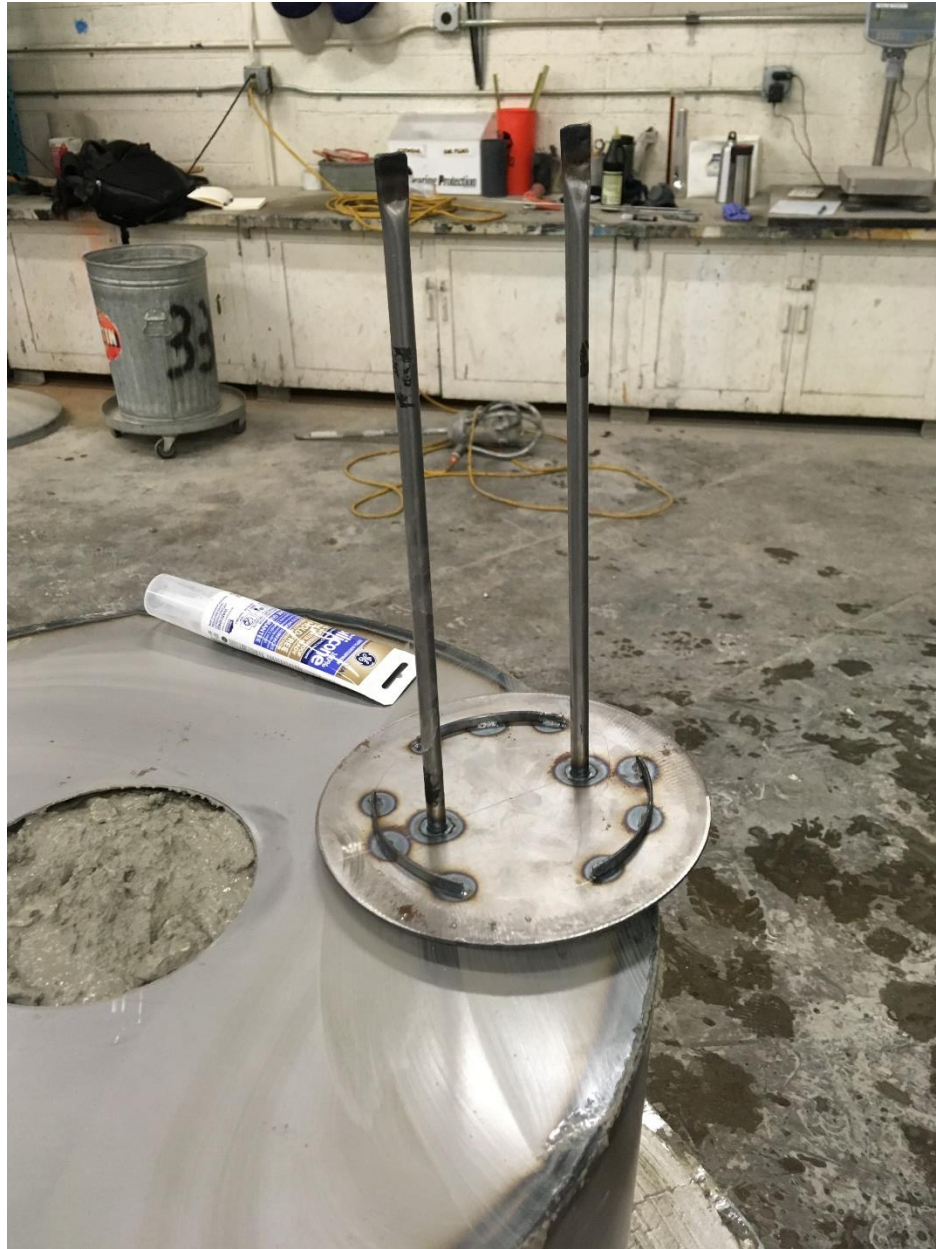
Figure 4-2: Picture of stainless steel plate with tubes attached that was inserted into concrete sample for thermocouple insertion
