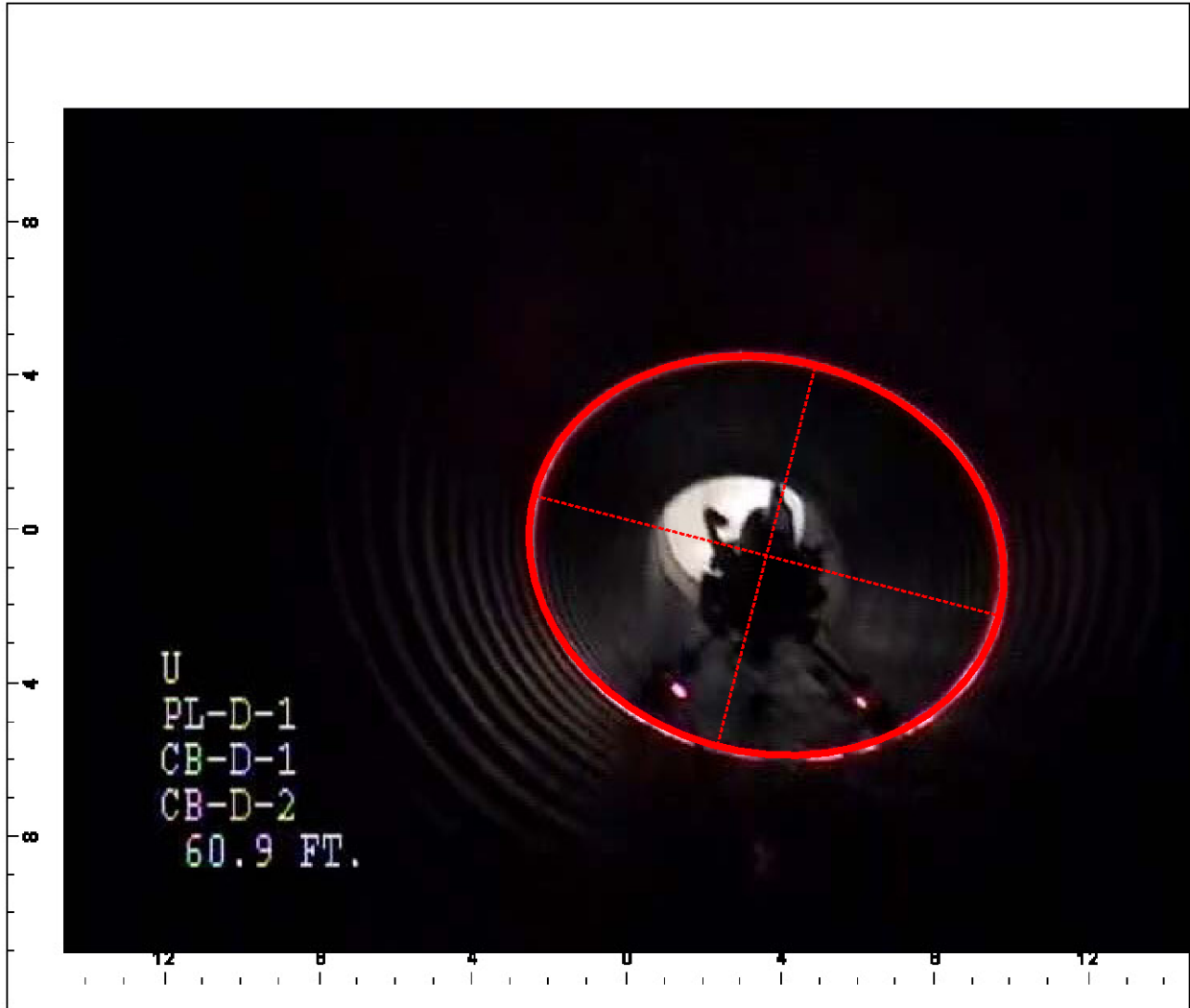
Figure 24 - Laser ring profiler with superimposed best-fit ellipse
