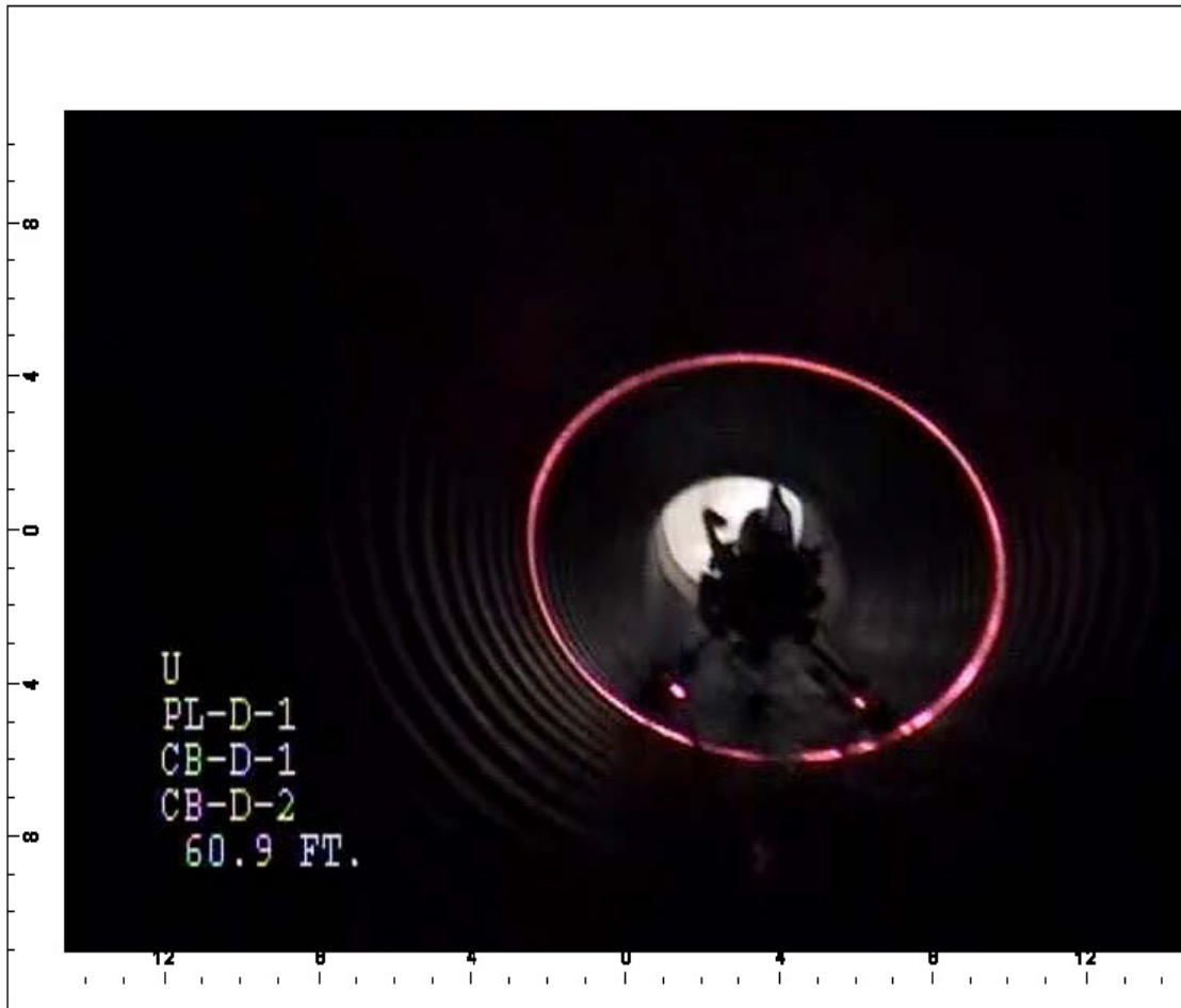
Figure 23 - Laser ring profiler cross-section
