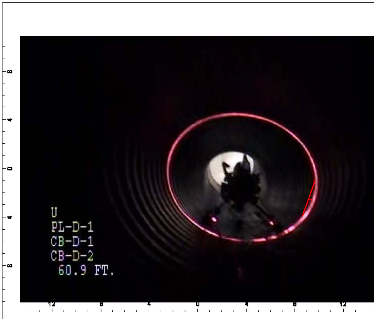
Figure 25 - Laser ring profiler with chord and sagitta
