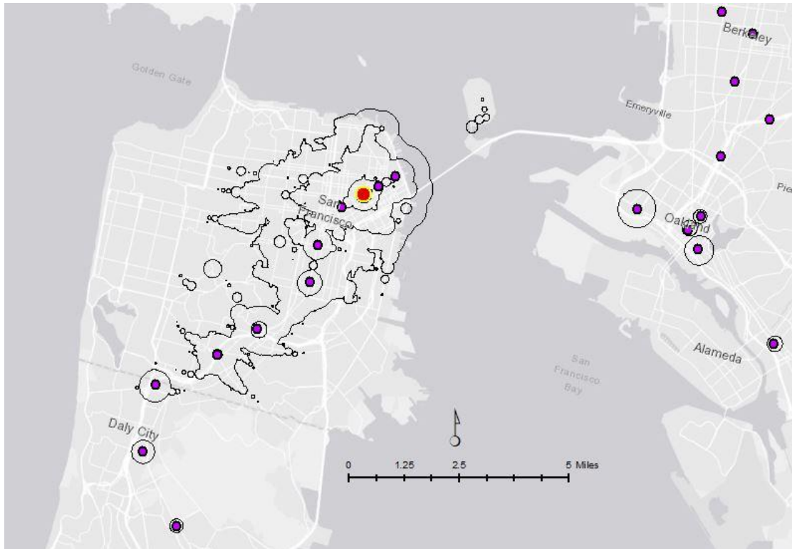
Figure 9. Example of a 30-minute job accessibility isochrones for the Powell Street Station (BART) in the San Francisco Financial District
