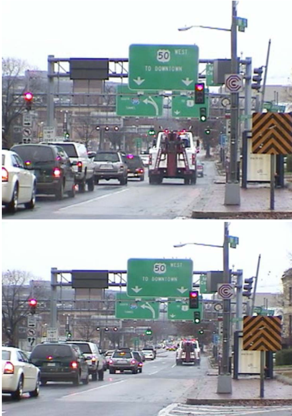
Figure A8-2 –Signal Layout along New York Ave at New Jersey Ave and Third Street may cause confusion, leading to red light running violations
