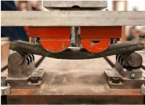
Figure 1. Ductile behavior of ECC material developed at LSU (6)
