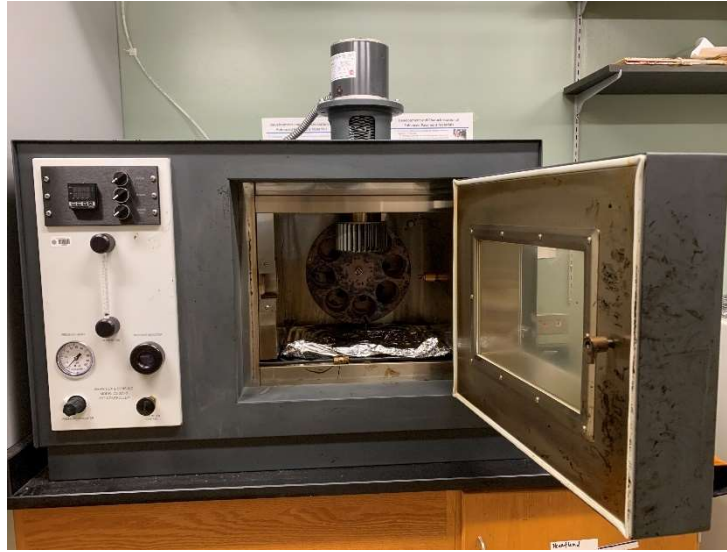
Figure 5: Rolling Thin-Film Oven (RTFO).
