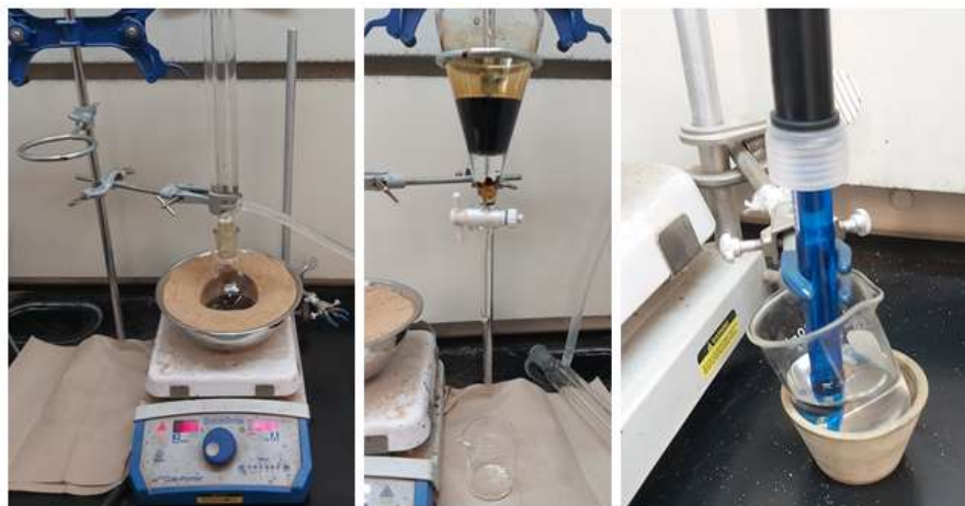
Figure 20: Acid number test: sample preparation (left), separation of aqueous layer from asphalt layer (middle), and measuring acid number (right).
