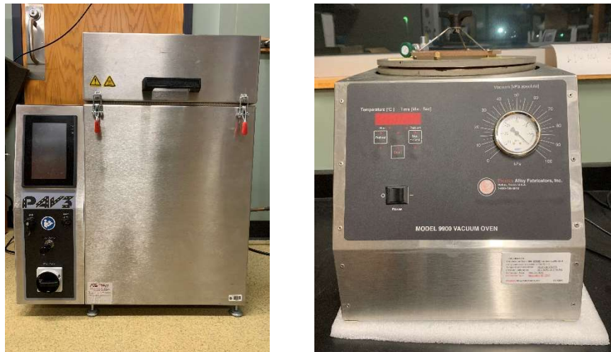
Figure 6: (a) Pressure Aging Vessel (PAV) (left), and (b) Degassing oven (right).
