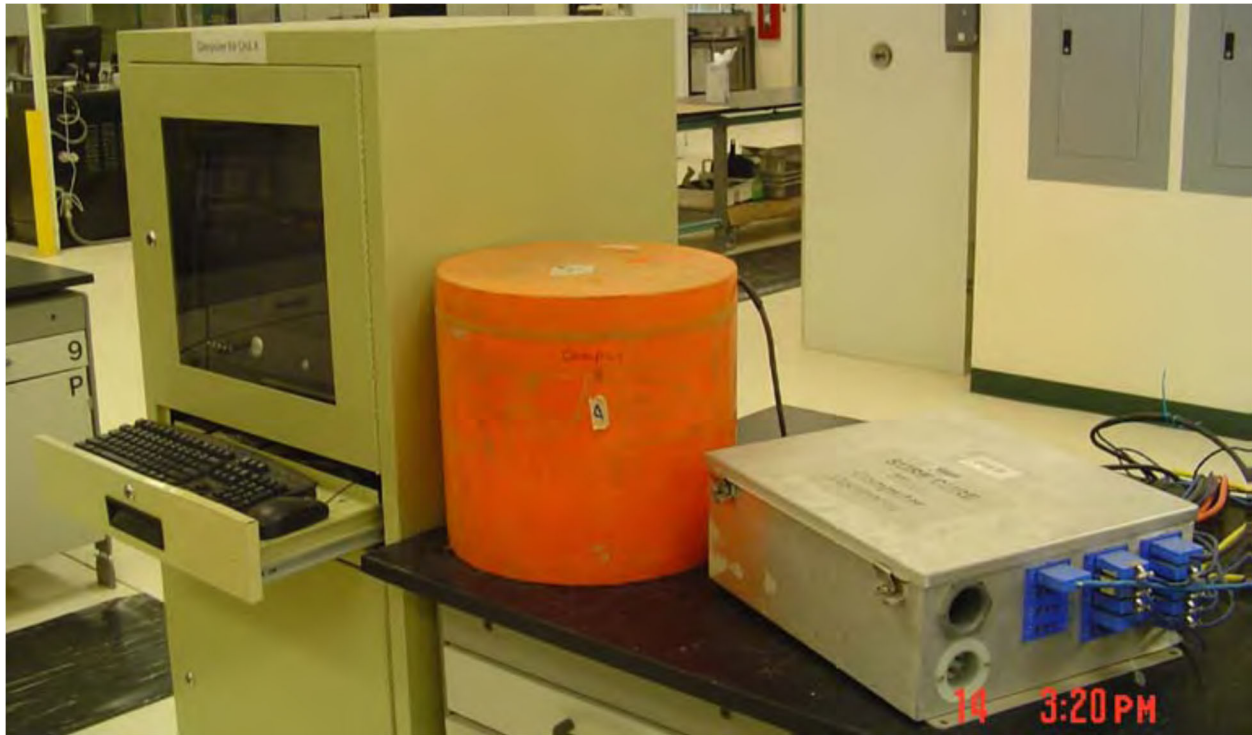
Figure 3. Sure Cure system with the computer, hydration chamber, and controller box by Products Engineering, Inc. [6].
