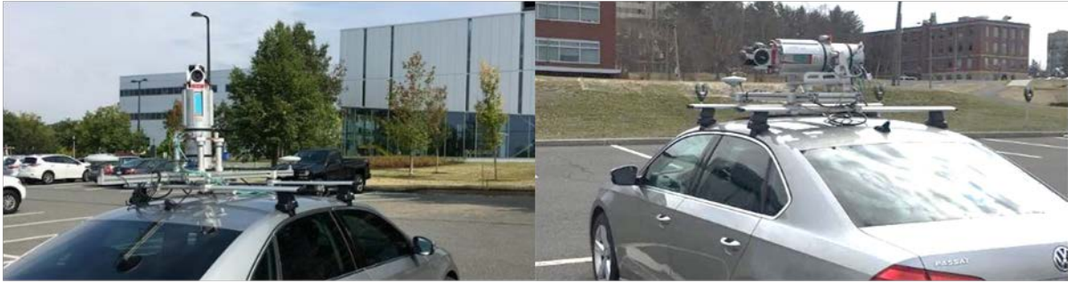
Figure 8 Mobile LiDAR installations for both vertical and horizontal configuration
