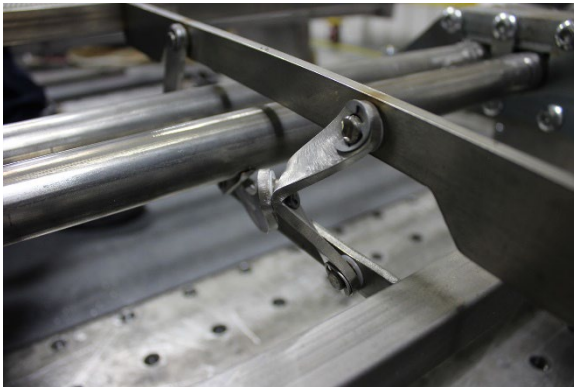
Figure 27: Test 2 Impact Seat Pan Structure
