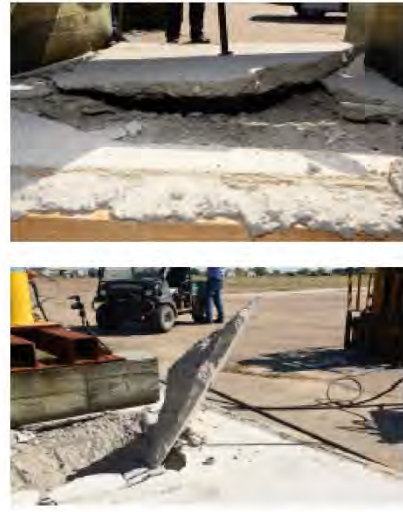
Figure. Cone-shaped failure observed in TTI test
