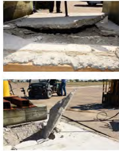
Figure. Cone-shaped failure observed in TTI test
