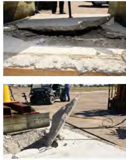
Figure. Cone-shaped failure observed in TTI test
