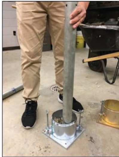
(a) Proctor Compaction
