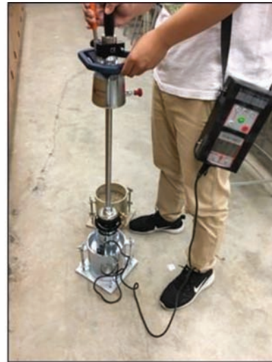
(b) LWD Test in Mold
