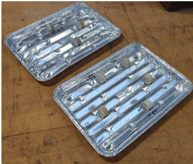
Fig. 40–Dry-out specimens in corrugated aluminum pans
