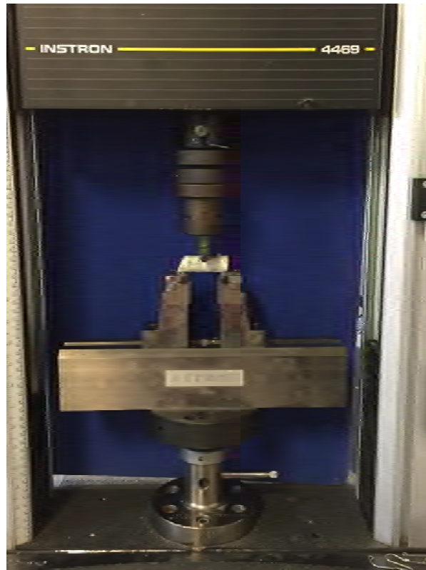
Fig 3. Short Bar Shear – Three Point Load Setup
