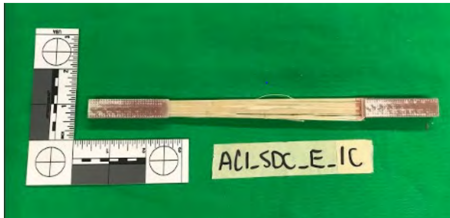
Fig. 7. Coupon E_1C after failure
