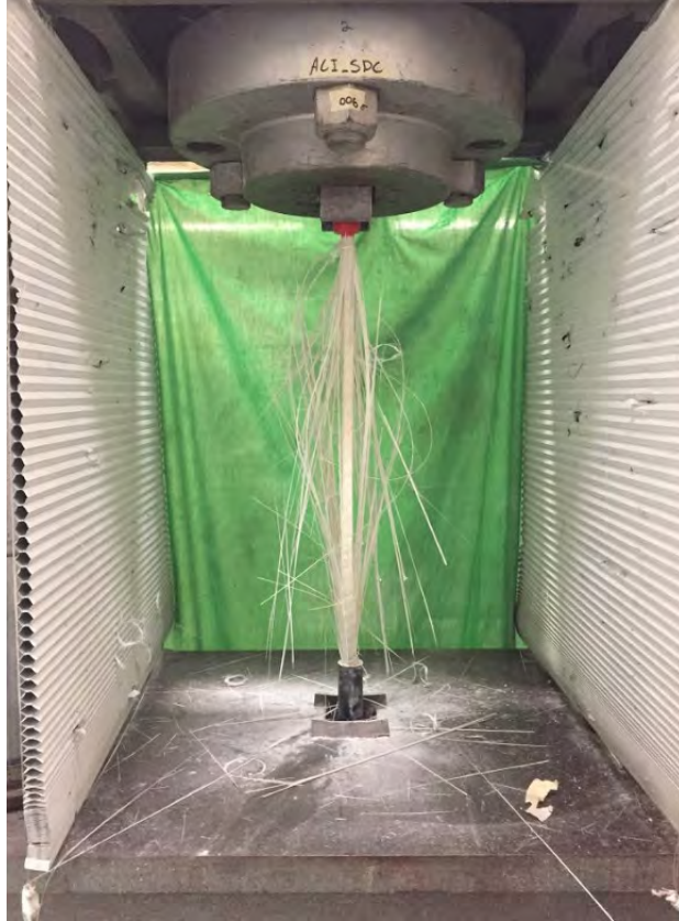
Fig. 60. Bar 006 after failure
