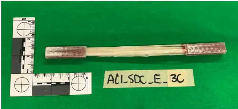
Fig. 25. Coupon E_3C after failure
