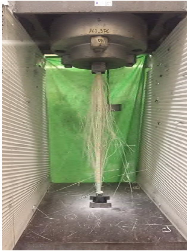
Fig. 54–Pristine GFRP tension failure
