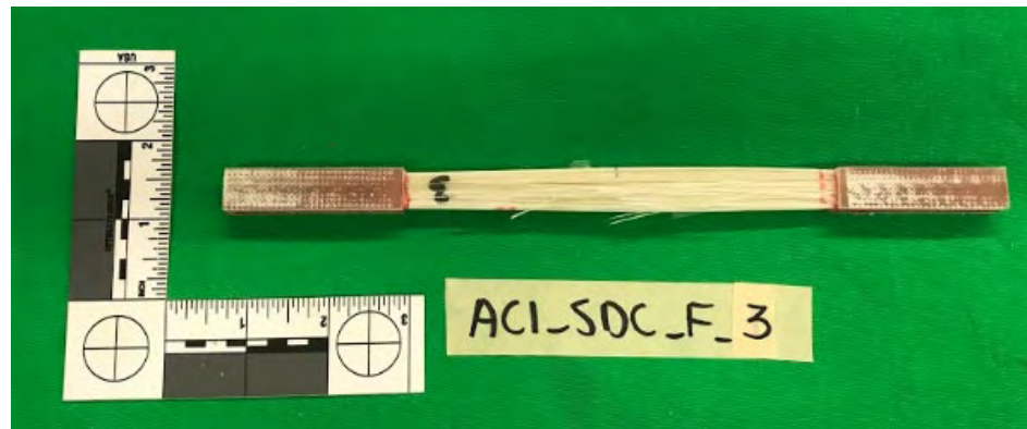
Fig. 35. Coupon F_3 after failure
