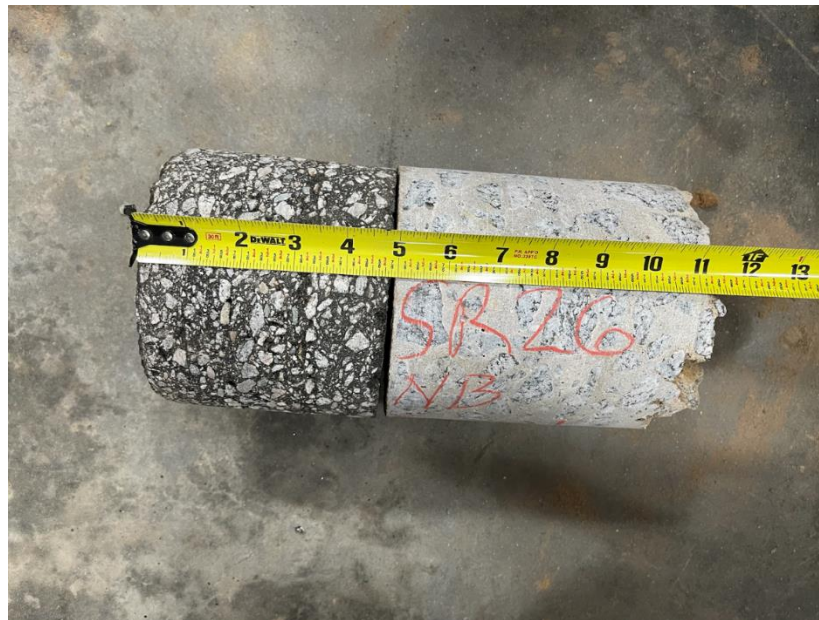
Figure 18. Photo. Composite Core 1 extracted from SR 26, featuring asphalt on top of PCC.
