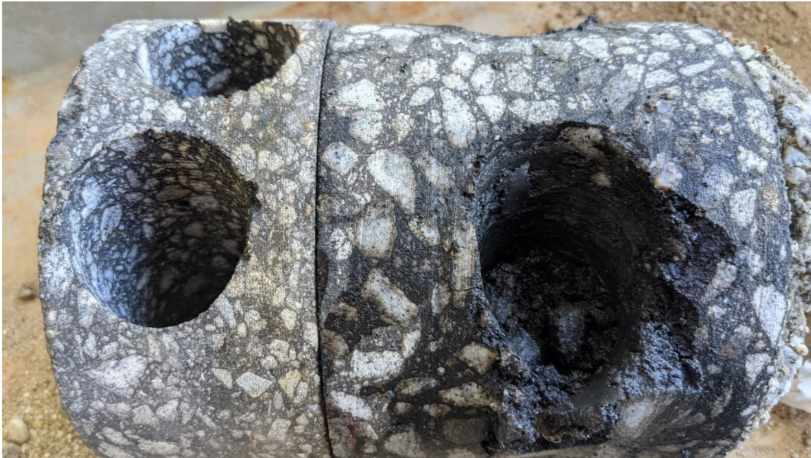
Figure 22. Photo. Asphalt core after 38 mm specimens were extracted for AMPT testing.
