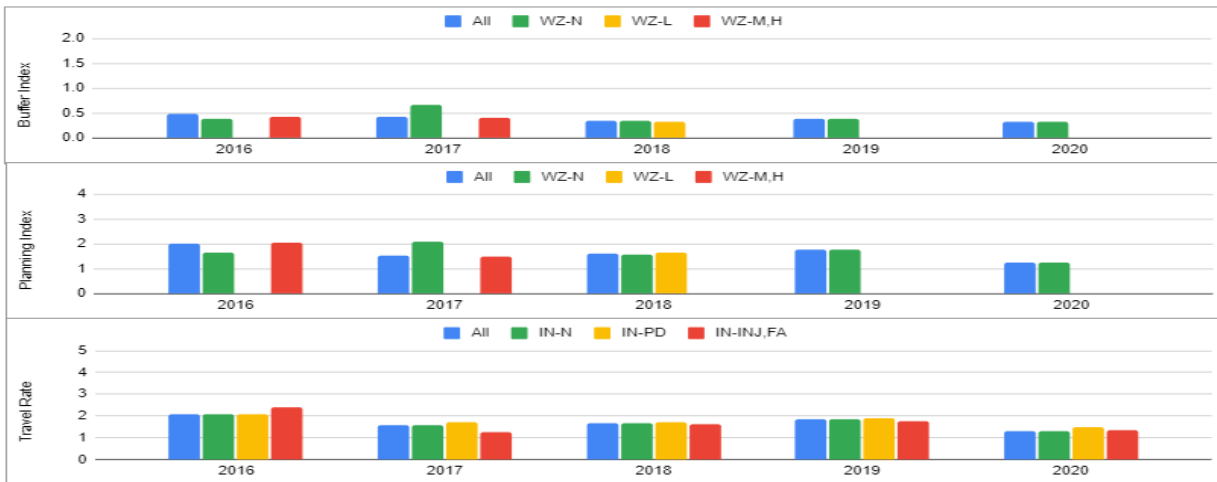
Figure 4.16: Yearly Variations of Reliability Measures under Different Work-Zone Conditions (169 NB)
