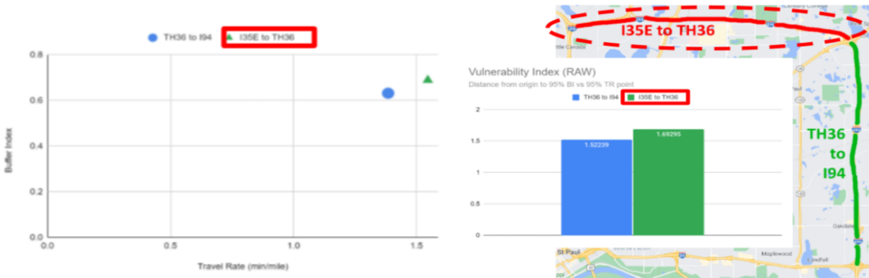
Figure 4.56: Identification of Bottleneck Sections (I-694 S1 EB)
