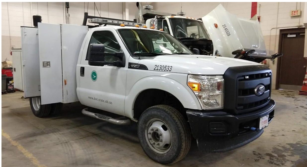
Figure 14. ODOT Licking County Garage mechanic's truck with passenger side tool cabinets open.
