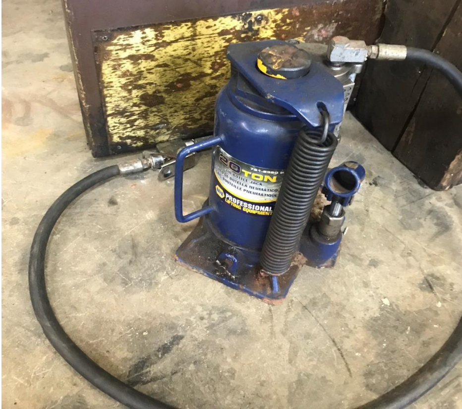
Figure 5. The hydraulic jack available for roadside repairs by the Pickaway County Garage.
