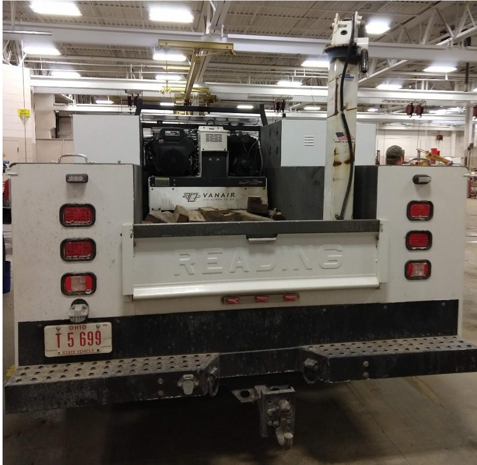
Figure 13. ODOT Licking County Garage mechanic's truck with built-in crane and compressor/generator unit.
