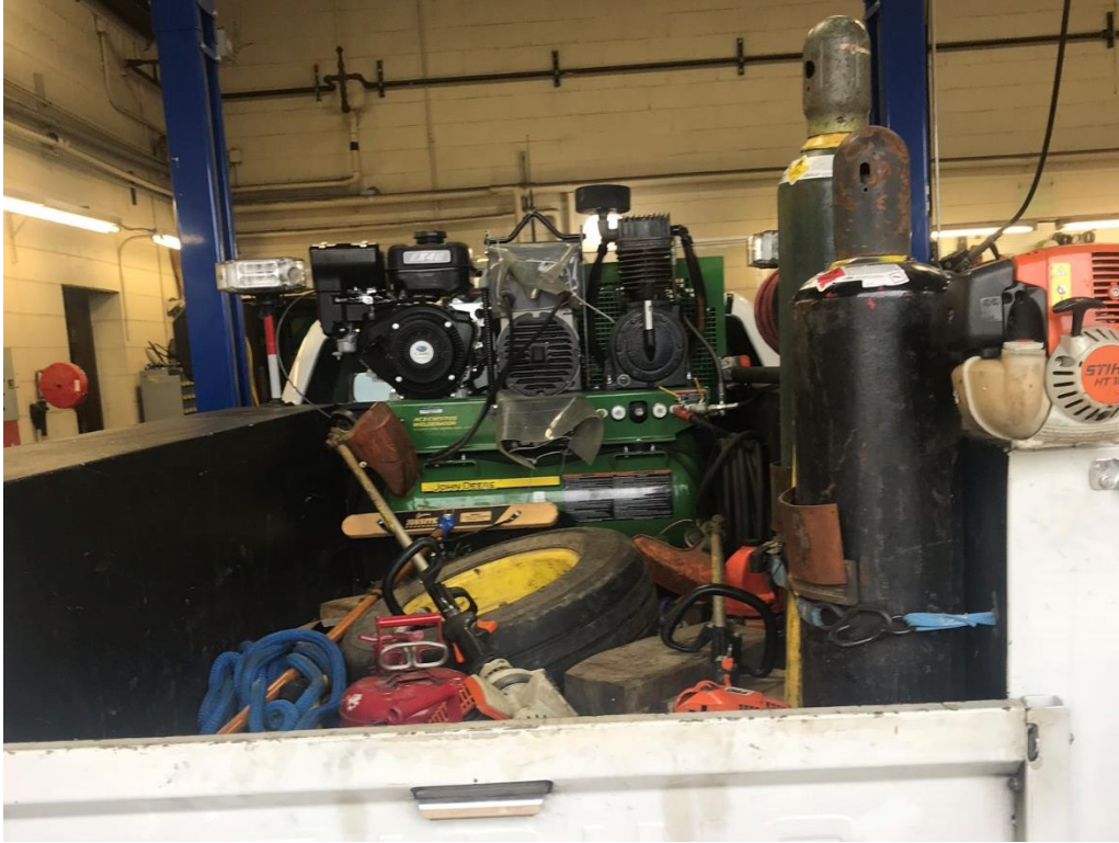
Figure 2. Air Compressor and Cutting Torches on the Pickaway County Garage Mechanic's Truck.
