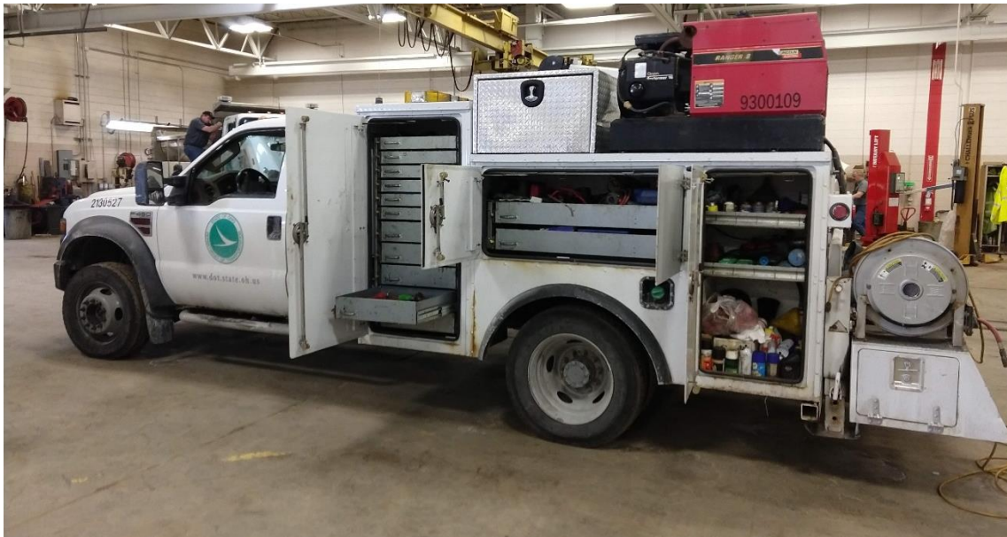
Figure 11. View of ODOT District 5 "Special Projects Truck" showing driver's side tool storage.
