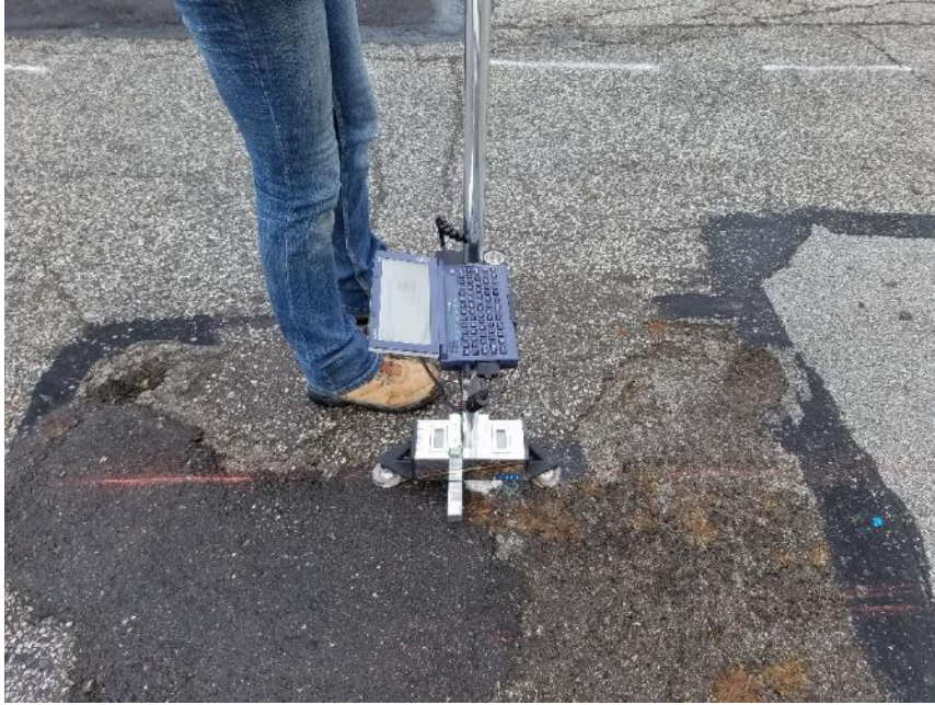
Figure 4 FACE Dipstick profiler used to collect profile along center of the lane.
