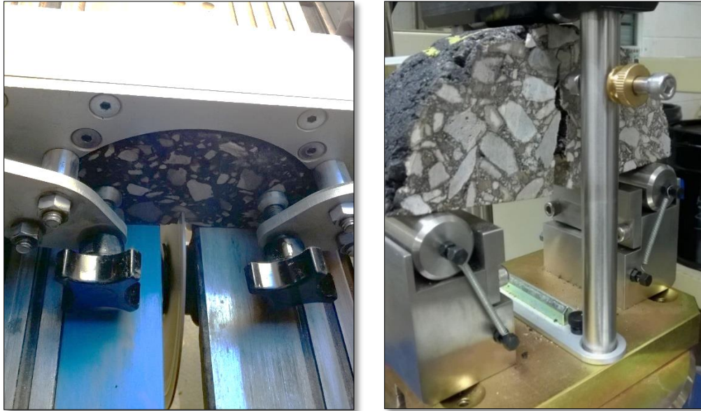
Figure C.3 Illinois SCB Sample Preparation and Testing Equipment
