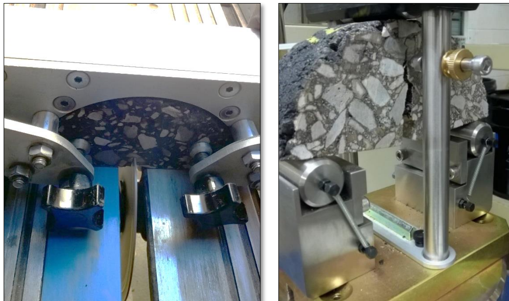
Figure A.3 Illinois SCB Sample Preparation and Testing Equipment
