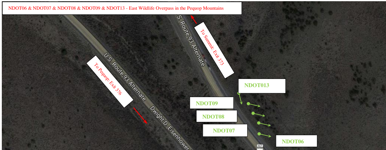
Figure 2-13 Cameras layout at the East Wildlife Overpass in the Pequop Mountains (2018 fall)
