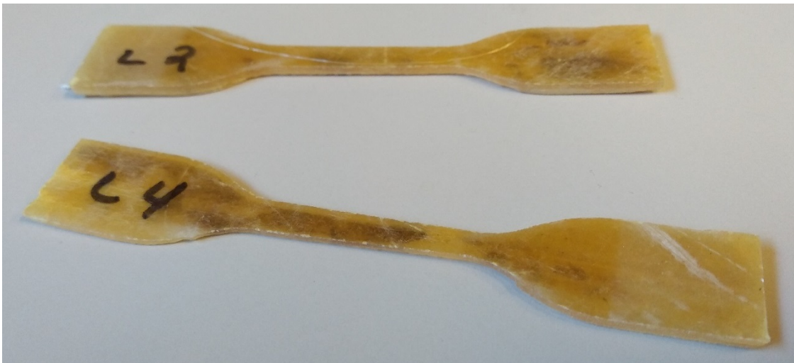
Figure 45. ASTM D638 Type IV Dog-bone Fiber-Reinforced Polymer Specimens
