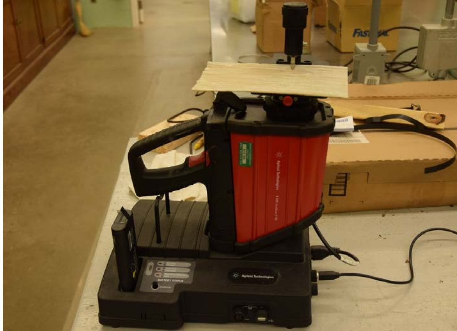
Figure 3. Fourier Transform Infrared Spectroscopy Equipment
