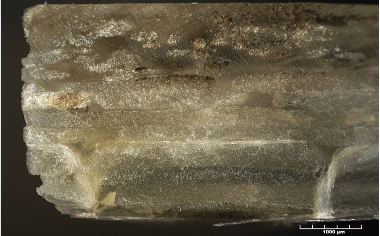
Figure 39. High-Resolution Optical Imaging of Polished Fiber-Reinforced Polymer Specimen
