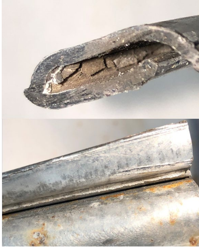
Figure 3.5. Coating defects within the bends of a lock-seam.
