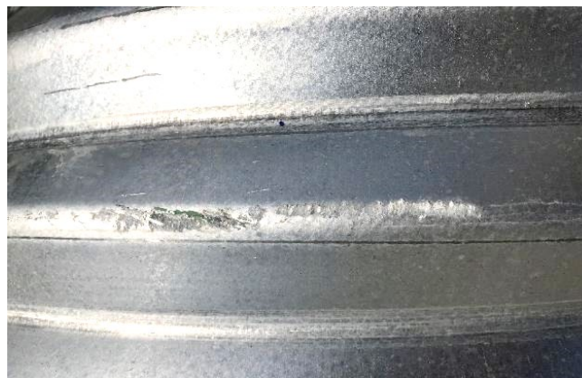
Figure 3.12. Common scrapes in the lock-seam and the corrugations of galvanized steel from Plant B.
