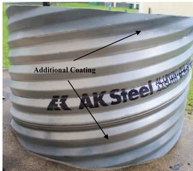
Figure 3.20. Additional spray-coated pipe in an aluminized steel pipe from Plant D.
