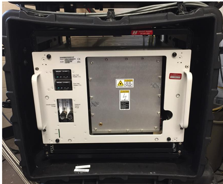
Figure 1: Marinerized MKS 2030 Fourier Transform Infrared Spectrometer (FTIR).
