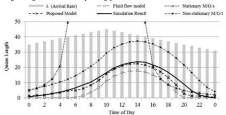
Figure 4. 2: Estimation result of each model in the numerical experiment (Source: Chen, 2014)
