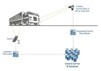
Figure 3. 1: OCR Technology (Source: kritikalsolutions website)
