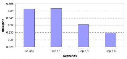
Figure 4. 14: Effect of Capping Truck Entry on Crane Utilization (Source: Huynh et al. 2005)
