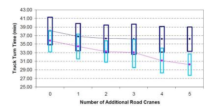
Figure 4. 12: Truck Turn Time vs. Additional Number of Road Cranes. (Source: Huynh et al. 2005)
