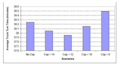
Figure 4. 13: Effect of Capping Truck Entry on Truck Turn Time (Source: Huynh et al. 2005)
